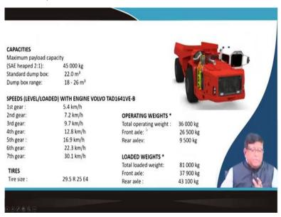
So, you have got these machines of very high capacity machines. You can see here the specifications that are the heat capacity is 45000 kg. That you know about the capacity of these are of dumpers are given by the society of automobile engineers specification. They give as a stuck capacity and heap capacity. Stuck capacity is just like when you fill a glass full of water at that time it is called your stuck capacity up to the brim.
