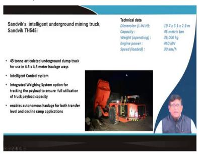
Now, you know that this machines it has got a number of features, particularly that in operating in underground mines its dimensions should be small. At the same time when it is a hard rock, the density of the material is high so that is why the total weight will be coming more. So, in a low height to accommodate nowadays even up to 21, 30 tonne they can be taken over this machine. So, the most important is how you will be powering this machine with engine.
