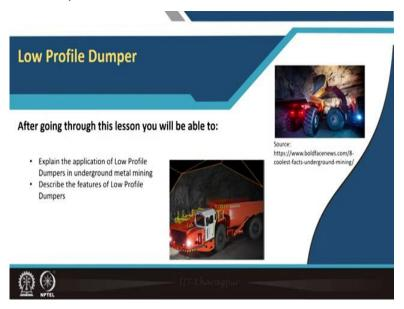
This low profile means that it is its height is lower so that it can work in a very confined space. So, you can see in that figure a dump truck which is of very low height so that it can work in the galleries of a underground mine. So now, in an underground mining, this conditions there is a biggest problem, is manoeuvring the equipment. That is why, as you can see in that figure, this type of truck which is having a box for dumping this box.
