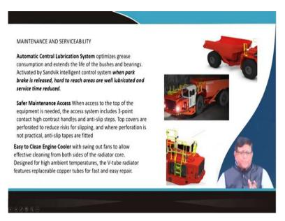
Then, maintenance and serviceability of this machine is also very important. So, to make it the so that the machine the designed in such a way that it has got automatic central lubrication system. Now, the lubrication is a very very important thing in any machinery because if the that do not do a proper lubrications, the heat generated may give a seizer and then your the parts get damaged.
