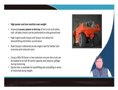
So, this machine is always a high power and low machine own weight. The there is a the materials which are used for construction of the chassis and the body and the parts they are selected in such a way that the self weight of the machine is less. So that it can carry maximum material by that this productivity is increased. And that you have seen in the previous one, that this machine, there are certain this components are given.
