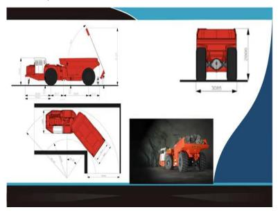
So, that that is why the power calculation that is what will be the driving power up to 450 kilowatt. Now, here in this figure, you can see the how operation that is your dimensional things is there? So, that you will have to make the select a machine for a particular mining condition making it compatible to operate over here. As you can see here, in an underground mine or in a tunneling operation, the tunnel, it is giving a you are having a semicircular opening.
