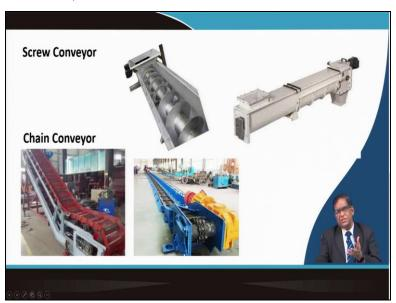
Similarly the other thing is the screw conveyors in plant that material can be transported by screw just like a auger takes off the wooden material from a wooden when you do the ordering see the same principle the screw conveyors can work. Then there are the chain conveyors used in underground mine bulk material handling quite a lot.
