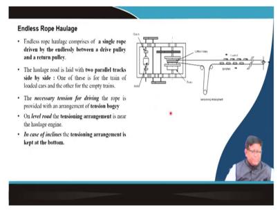
The other one is a endless rope haulage, in the endless rope haulage the system is your one rope. This exactly you can see the rope here it is going over here and it is connecting over there. This is a clifton pulley, a conical drum type of a pulley in which this rope is taking a turn and it is going over here. There is this rope will have to be kept under tension. That is, if the tension is not there, the power will not be going to this or that rope will not be driven.
