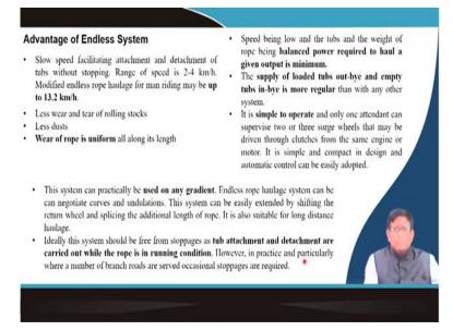
So, the advantage of this system is its slow speed, facilitating attachment and the detachment. That means it will be moving at a speed from 2.4 kilometer per hour at if your man riding system can be used because there you will once it is connected, you will not be disconnected only up to the end you will be going and you can make it up to a speed of 13.2 kilometer per hour. And there the rolling stokes they get less, wear and tear.
