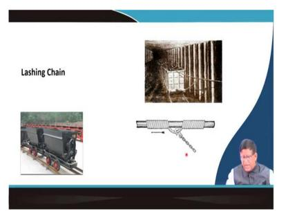
And the lashing chain you can see that this chain is the lashing chain and that chain will be coming with a clip is there on the rope it will be connected. And then you can usually this will be moving that where rope is moving and that this at you and you can lash it with that car mine car will be having this type of lashing chain.
