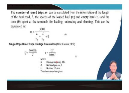
So, what once you know this then you need to find out how that m, your for this, the number of round trip per hour? How many trips it will make in an underground conditions? It can be calculated from what is the length of the hole? What is the speed of the loaded hole and the empty hole? That is your loaded will be going at a different speed say v L and the empties are going with a v E and then if it is total time theta that has been spent at the terminal and for loading.
