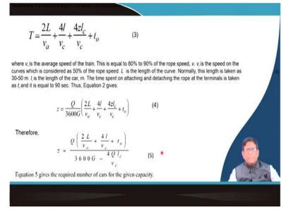
So, this type of calculations can be carried out by this simple equations. That this time which we are taking that is your the if your total time required here as say your this total time will be the main factor that is the for the whole productivity calculation and this is calculated by knowing that that is your the velocities that speed that is, average speed of the train and then when it is carrying out that is your the at the curve.
