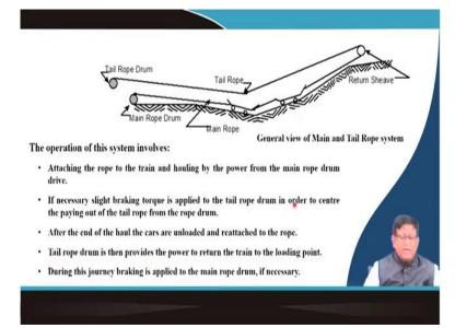
So, there will be more load will be coming over here this is a bigger system. So that means you can arrange the main and tail rope in a different way. In the underground mine you can think that this is there inside the mine. How you are doing there is a your tail and drum is connected over here, main rope drum is connected over here then your this will be the tail rope will be going.
