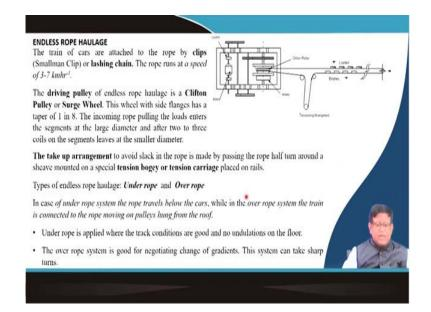
Then the main cars are attached to the rope bike clips. That is a your rope which will be moving over here you will have to clip it. So that it can go on moving over there. And when you are to take it out from there you remove that clip and then your rope will be free you can bring the empty and you can connect it over there. So, this there were the lashing chain and this small man clip there was a in that old days.
