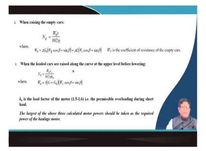
That is when raising the empty cars and when loaded cuts are raising along the curve. So, under these three conditions, you can calculate out the total power required. And your normally, this factor which is you, are keeping as a load factor 1.5 to 1.6 as a for overloading you will have to do it because while calculating in mining operations, you always see that the factor of safety is always taken at a higher.
