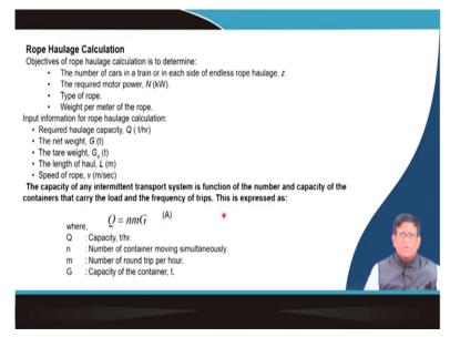
And once you have done these things, try to draw the drawings of them you will be able to know. Now, when you are to do some calculation of this. The objective of the rope haulage calculation is to determine that what is the number of cars in a train or in each side of the endless rope haulage? How many number of cars you will be connecting that z, calculating that is a one issue.
