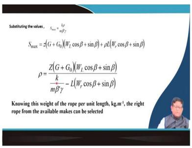
So that means the from the knowing this maximum tensions over here. And then, when you will be knowing what will be the your weight of this that is your the per meter rope weight because this will be ultimately contributing to what is the motor power required. So, knowing this rope the weight of the rope per unit length, the right rope from the available make can be selected.
