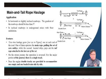
So, what is the main and tail rope haulage? In our direct rope haulage, you have seen that there is one drum and that are being brought. Now, here you can see that is, there is a main rope with a main your drum and there is a tail and drum with a tail rope. That means your that mine cars are forming a train, the end side and front side both side a rope is connected. So that is your exactly main and tail rope system.
