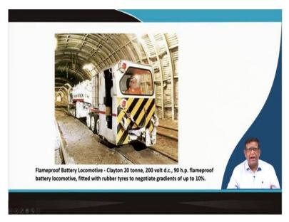
And then you can see that this battery locomotive it will be even in a gassy mine, with a flame proof battery enclosure, they can work such type of things in the underground mine can work.
