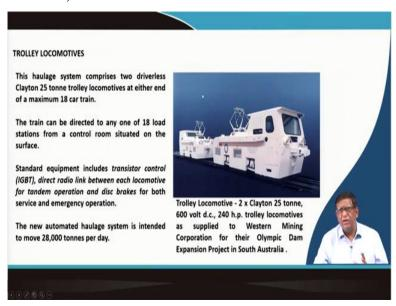
There could be a trolley locomotive that this locomotive they are having in underground mine. There could be electric line going on if it is not a gassy mines. It is in a metal mine, you can have a this type of transportation system.
