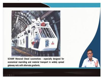
You can see here how it in this is a mono rail. On that, this trolley is suspended and with the battery it is just going on running these things. The whole thing as a train you can collect at the back. It will go either for man riding as well as for material riding.
