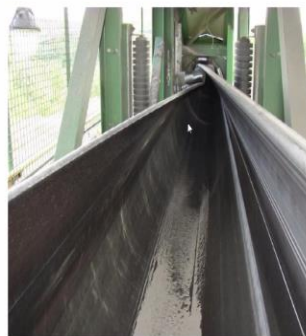
Folding belt from flat shape into a pipe shape. (M.E. Zamiralova, G. Lodewijks, 2015)
