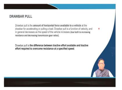
Now, this concept, as I said that drawbar pull whenever you talk of a dozer whenever you talk of a this scraper whenever you are talking of a tractor whenever you are talking of any this your towed vehicle the drawbar pull is the amount of horizontal force available to a vehicle at the drawbar that where it is getting connected for accelerating or pulling the load. So, all your side discharge dump trucks your the that your rear your bottom distance dump truck.
