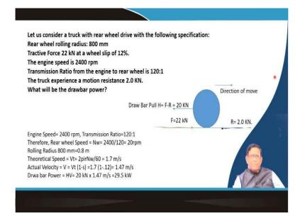
Say let us consider one truck with a rear wheel drive which the following specifications. A rear wheel rolling resist radius it is say 800 millimetre, that is your the radiate rolling resistant from here this radius is 800 millimetre and the tractive force is 22 or we say I thought that this is 22 kilo newton it is your because this direction it is moving in this direction. So, that is your tractive force is giving 22 kilo newton.
