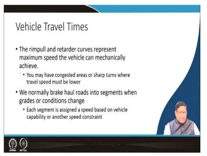
So, then once you know these things that from the speed you can find out what will be the travel time. The Rimpull and retarder curves they will represent the maximum speed the vehicle mechanically can achieve. So, you may the that have the congested areas or sharp turns where the travel speed must be lower or under that conditions if some when in a mines you will be going from one directions.
