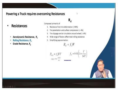
So, then other things; that which you will be requiring is the rolling resistance. Rolling resistance is the resistance which is coming from the tire and road interactions. There are different ways of calculating determining that in the field but we have not done much of these experimental determinations many a times we take the rolling that frictional the resistance that rolling friction.
