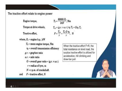
Because this is related to your engine power. That is how that engine will be used using that how the engine will be delivering the power to get the traction. So, you know that engine torque it is exactly what is the engine brake power given in kilowatt if it is P e and then your this the crankshaft of that engine crankshaft is giving a rotation of N rpm. Then this tractive engine torque you are finding it in newton meter as given in this equation.
