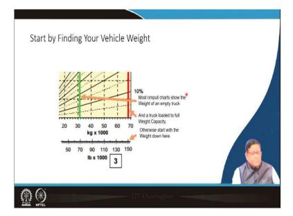
So, first what will have to do, what is your vehicle weight you need to find out. Now and then what exactly the for a particular vehicle when you get a Rimpull diagram, there will be one green line and one red line. This green line it will show that your Rimpull shows the weight of an empty truck this is this will give the weight of an empty truck that is here at 30 ton. And then when it is a full loaded because it is a 40-ton truck that means this is a 70 ton is the full load.
