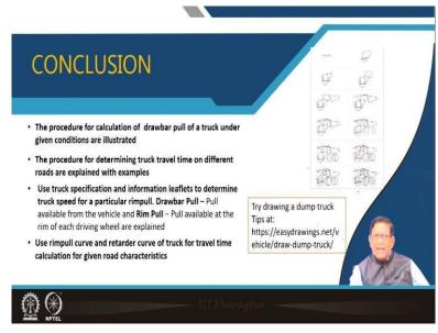
And then the procedure for determining the truck travel time on different roads it is just mentioned over here and the truck specifications and information leaflets you will have to use that thing for determining the drawbar pull. And that the drawbar pull which is the pull available for the vehicle. And the Rimpull is the pull available at the rim of each of the driving wheel that is we have just explained briefly.
