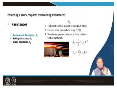
Now, you know that three types of resistances are very common when a that is it will have to be overcome and to overcome this resistances power will have to come from the engine. Now, these aerodynamic resistances it is the air resistance. Say for example you can see in that figure that when the truck is moving the air will be giving a resistance to it that is why whether the tire has got a, mirrors it has got a front size.
