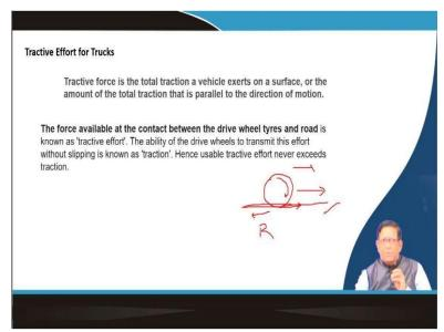
This is another very important thing that what is attractive effort for a truck or the attractive force is the total traction a vehicle exerts on a surface. That means when that engine is running at that time that your will which will rotate at that time how much exactly the vehicle can be propelled, how much it can be tracked that is the amount of the total traction in is in the parallel to the direction of motion.
