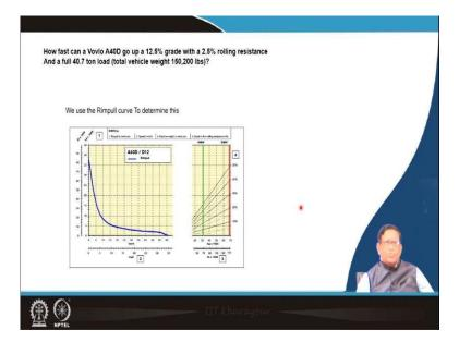
So, then the other things which you need to know. Suppose here I am showing you one curve it is called your Rimpull curve. All the manufacturer they give that is for their machines they do experimentally determine and they provide this their Rimpull curves. That means how much exactly that pull or the force will be available when the car will be moving at different speeds. So, in this one you can see the speed is given and in this here the your pull is given.
