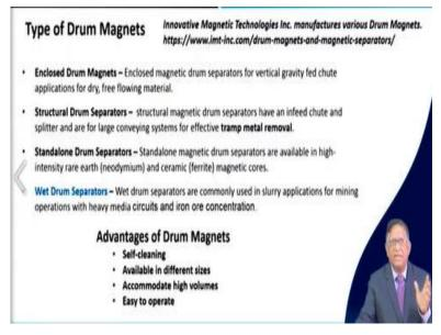
Now, there are different types of drum magnets. There are different companies you can see the websites of the manufacturer to find out over here. That drum magnet may be your enclosed type of drum magnet. There are structural drum separators and then there are standalone drum separator and wet drum separators. Out of these your enclosed drum separator that is your enclosed magnetic drum.
