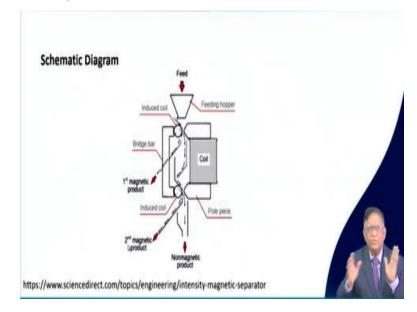
So, how that schematically if you see that in a WHIMS or in any of these magnetic separations your feed is coming over here and there is your induced coil your generating a magnetic flux over here. When it is going the magnetic particles which have got strong magnetic property, they will be getting attracted to this and through this chute they will be coming out. They have got the first magnetic product. Now then the material will be going through another.
