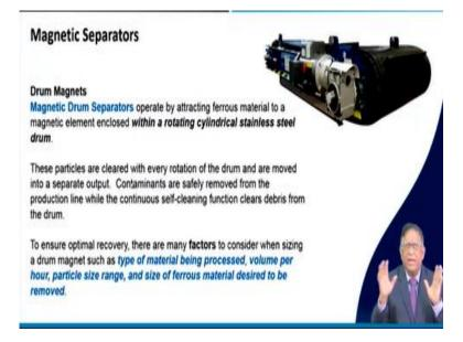
And then there are different companies they manufacture this type of devices. Now as a magnetic separator there we say is a drum magnet exactly this drum or that your end pulley that will be considered that will be made a magnetic thing. So, that is then we are telling it as a magnetic drum separator. They are attracting the ferrous material to a magnet element enclosed within a rotating cylindrical stainless steel drum. So, there inside they keep it.
