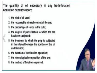
Now the quantity of the oil necessary in any froth flotation operation depends upon number of factors. That is what kind of oil is used? The recoverable mineral contents of the ore then the percentage of the solids in the pulp, the degree of pulverization. I told already the how much the quality of grinding. The treatment to which the; pulp is subjected to in the interval between the addition of the oil and flotation.
