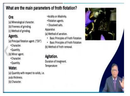
Now the overall that when you are doing this operation of forming the froth and adding oil and things like that you are controlling you need to consider different parameters which are related to the ore. Their mineralogical character, their fineness of grinding, and their method of grinding depending on which method you have made it whether it is autogenous mill only, whether it is a ball mill, whether it is a rod mill they will be giving different characteristics of the material.
