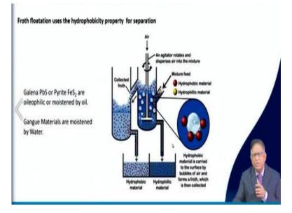
So, in the whole process of froth flotations there are different types of the systems are exactly you can design depending on the plant size depending on where it will have to be accommodated. What is their location with the other processing lines? Then the design will be done in the plant design. But basically, as a component wise how it will be there? You can think of with this diagram that is if we are doing this or mainly for the hydrophobicity or this oileophilicity.
