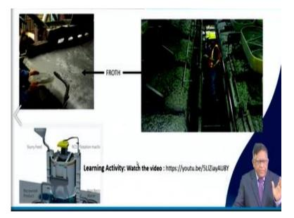
Now you can see that in real life if you see how the froth is coming? That is from there this is flowing over this they collect the froth. Test it whether the things required reagents and all are given properly or not. There could be number of chambers the froth is getting formed. Now the efficiency of the system performance how it is performing? Whether any valuable minerals all are coming into this froth or not. That will be depending on number of operating parameters.
