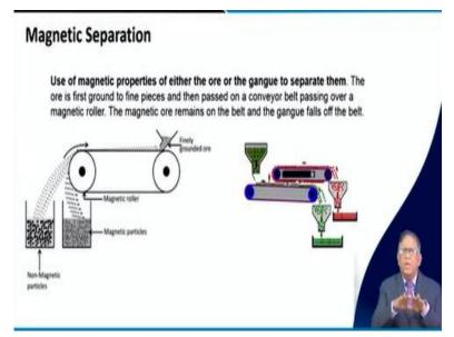
So, then we are switching over to another system which is our magnetic separation. This also I told you earlier that the magnetic separator it is done. We can do it in the wet form or in the dry form when the materials are moving. At that time if your feed material has got the magnetic property magnetic susceptibility magnetic that is say it can be attracted by magnet. Under that conditions you can use this system.
