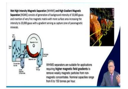
Now this wet high intensity magnetic separation that WHIMS or that the high gradient magnetic separation called HGMS. These two are the techniques which are as an advanced technique they have been used in many sulphide ore beneficiation. Now you can see here that is the intensity of about 10,000 gauss of that is your magnetic intensity you will have to create. That is one gauss is 10 to the power minus 4 tesla.
