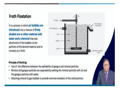
The froth floatation is one of the oldest techniques and it is being used in the processing plants of various types of ore particularly wherever we are having the sulphide ores or even in some of the other minerals also. But there are whether to separate out in the froths. The mineral ore we are separating out the gangue material. So, this process basically it involves that is you introduce air bubbles.
