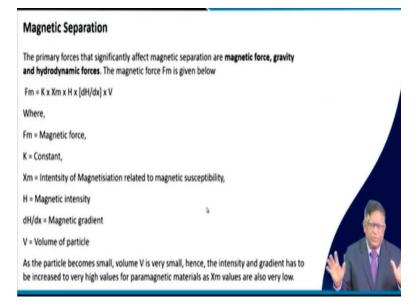
Now what is the basic principle of that magnetic separation? That is the magnetic force that is how the gravity force and the hydrodynamic force all these forces they need to be analysed for seeing that how much exactly the magnetic force will be required to separate that out. Basically, this is one of the very common equations you will find where this magnetic force this is exactly related to it K here is a constant and then this is your intensity of magnetizations.
