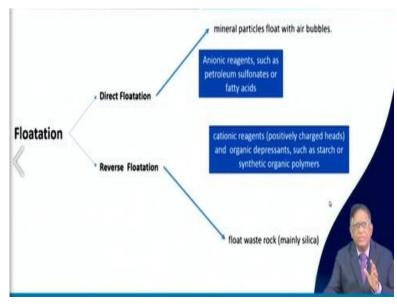
So, this is how but we have this floatation system as 2 type. That is direct flotation or reverse floatation. In the direct flotation your mineral particles they float with the bubbles. So, this is what is happening? Mainly the anionic reagents such as your petroleum sulfonates or fatty acids when they are put it over there, they will attract those things and it will be going. And then normally what happens?
