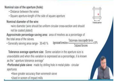
Now what is done in sieving? Your nominal size or aperture of the sieve or the screen shape. This is given by this one. Now the distance between the wires is called the nominal aperture. Now when you will be doing the calculations of how that sieving will be performing because these wires are also occupying some space that will have to be taken care of. Now the nominal diameter of the wire depending on that your screen performance will also change.
