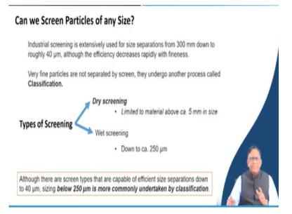
Then in your screening operations in the industry in a mineral processing plant will you take it for all type of materials. Normally it is not. You will be having always working within a range. So, normally that 300 millimetre 30 centimetre and down to 40 micron this is a normal. But depending on that you can have tailor-made machines creation is not at all a problem. Provided if you have got to give a properly whatever you need it can be done.
