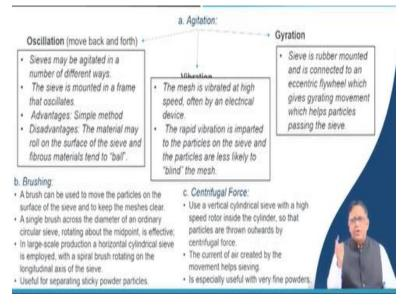
Oscillations that is your sieve will be giving all the time oscillating like that. In a vibration sieve will be given a vibration like this. Then the gyration sieve will be rotated like that. Brushing means with a brush you will be going on handling over there. And then in a centrifugal force
