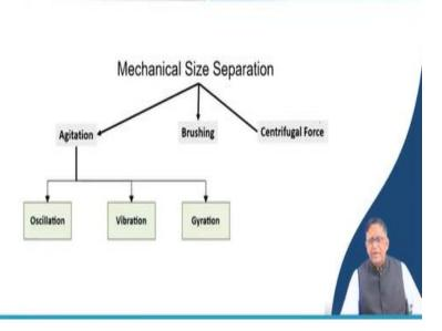
So, this will be very interesting when you will be working in the laboratory. Normally in the bulk material handling laboratory you do this analysis. Now it is exactly that how you can do these separations? That can be by agitation, brushing and centrifugal force for the finer particles. That vibration or that agitations for screening it can be given by oscillation, vibration or by gyration. For the sieve analysis also, you will have to have this system and that can be done over there.
