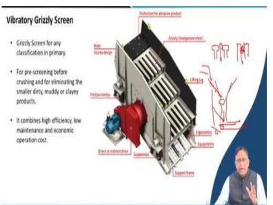
Now, you can see here there is a vibratory screen that can be of a grizzly type. That a grizzly types of screen it can be vibratory or it can be static also. Now what is the grizzly? Grizzly is just you can see here. These are very manganese steel rods. You can see over here which are having it is normally a T section. At the top it is wider and then the below it has got a less thickness. So, that if any rock mass if it go over there.
