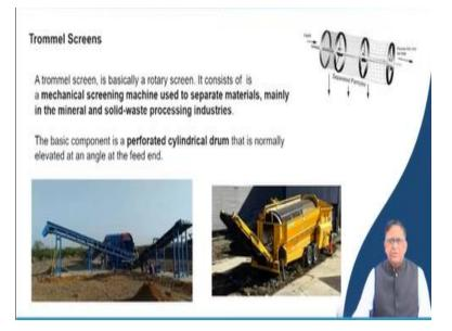
Now you may be seeing some of the screening operations of different type of bulk material say in our municipality waste from there when you want to do that is also a screen which is a trommel screen. We also use in the mineral processing sometimes separating some of the coal particles. There also we have got a trommel type and in which the whole crushed coal will be given. The trommel will be rotated and the finer that the small size coal will be taken out.
