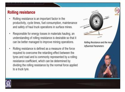
As I was telling about the rolling resistance you know that that when a tire is moving over here that whole traction will be taking place because of the resistances over here. Now this tire has got those trades and this they will be running at a different speed. So, the rolling resistance which will be opposing the speed affects the things. So, there will be when will be discussing about the truck.
