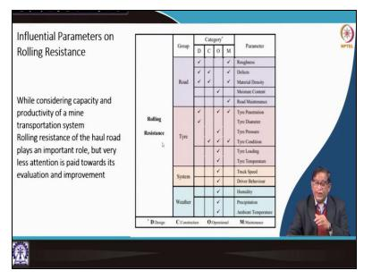
So, there are influencing parameters on rolling resistance that rolling resistance you have said. Now here I am giving you a tip that why you should be studying these things little bit more deeper that simple rolling resistance this can be affected by a that is we are considering the capacity and productivity but that rolling resistance can affect a number of thing that is exactly the road, tire, system and weather everything can be affected by the rolling resistance.
