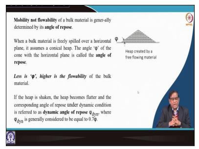
We have also talked about the angle of repose in last class once again to recapitulate the flowability that is your and mobility these two are the different things. So, that is which are exactly determined by angle of repose when you keep the material as you can see here if you pour the material from top it will take a shape like a cone like this. This angle it is called the angle of repose.
