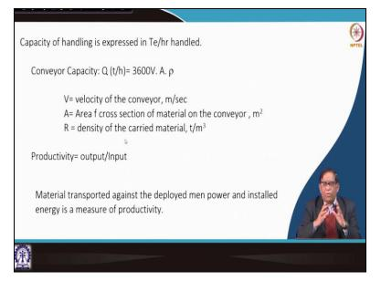
So, normally when we talk about the capacity it is that your carrying capacity that means how much is the conveying capacity. If your say on a belt conveyor if your velocity of treble is a v meter per second and then area of material on the cross sections of that cross section of the material on the conveyor belt is A and if that density is rho then your simply you can calculate how much is the tone per hour taken.
