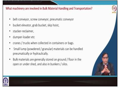
So, these are the some of the things you should do it then what machinery are involved in the bulk material handling you know already in the first class introductions I have said the belt conveyors screw conveyor bucket elevator sticker reclaimer dumper loader crane truck then your you have got number of pneumatic and hydraulic transports you have also sometimes been bunker silos for storage will have to be studied.
