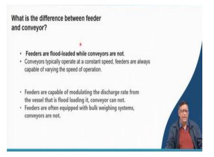
So, the basic difference between a feeder and a conveyor is then feeders are flood loaded whole the material come over there and they will have to be high torque must be applied for driving it. In a conveyor belt it is just a loading is not by the head load is not there. So, compared to the feeder they may have a low power to supplement.
