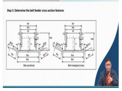
And then in this skirt board the front side what will be that these dimensions will have to be created that is your whether that built. That is the total belt length and then the belt will be sometime if it is shifted. Now then the whole system will be different. So, here you can see the belt is having a centrally running. So, under different conditions your feeding load will be different. So, this is just for your understanding we are not going to the detailed design over here.
