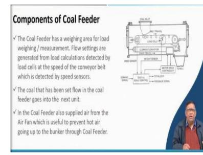
Now what is there in a your coal feeder? If you can see here one thing is there very much that is the components you can see one conveyor belt is over here and this conveyor belt if there is any spillage and all there is a clean out conveyor belt this will take the material and again it will be giving it to be sand to the mill or wait it will be crushed for fine so that they are sending it to mill. Now what is there?
