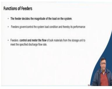
So, what exactly if we are thinking of selecting or designing a feeder, we will have to know that what are the functions it will have to be it will do. The feeder decides the magnitude of the load on the system that is how the load will be taken on to the feeder so the total the conveyor belt and all how it will be loaded because you are regulating. How, much material you are loading on to the next conveyor belt depending on that their power will have to be decided.
