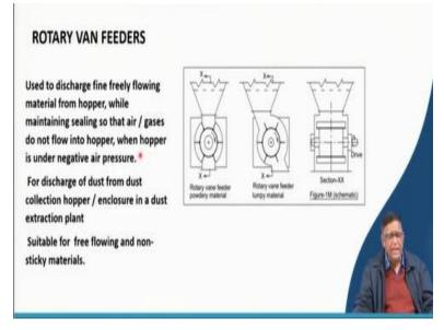
Then the van feeders that when this is a drum it is rotating over here, these vans are there so these vans come out so in this portion the material gets stuck. So, whatever the material is coming it is guided through this and then it is coming out.
