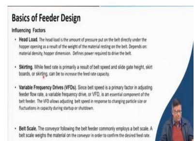
So, while you are going to do for this design, the influencing factors are the head load, skirting, variable frequency drive for giving your variable speed and the belt scales. As I have shown that these four things the head load is the total load which is coming on the feeder. Because of that this is in the conveyor belt design their force gates this head load do not come. But in case of your feeder design, you will have to do head load.
