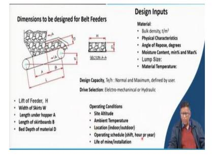
So, you can see here in a design of a feeder you will have to type find out these dimensions. That is your what is that your total length and then how much lift has been there and then if you see from front side that what is this width of that and then what is your exactly total under that hopper how much is in this portion, how much is in this portion this makes the whole design. And ultimately you will have to find out what is your design capacity and what is your drive selection.
