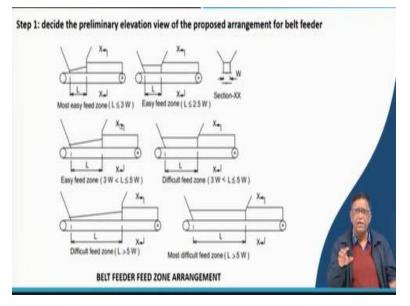
Now that zone which we are telling that means your belt feeder zones that where the belt is having a this much long of skirt board or it is having your this is the portion of the skirt board. Sometimes you may have a this whole material here if this L is longer here the material which is getting loaded on this d is also getting a velocity and coming over here and then put it. So, this different type of designs could be there.
