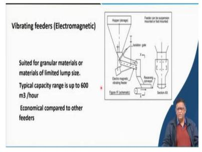
A vibrating feeder where the material coming from a hopper this portion is given a vibration by electromagnetically then the material is coming out of it and then loading into the conveyor belt.
