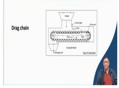
Then there is a drag chain. This is you have seen in a in some of the reclaimer of there where a chain is going and there are the flight bars. This flight bars will be pushing the material from here and it is going. In a scrapper reclaimer you have seen this type of system over there.
