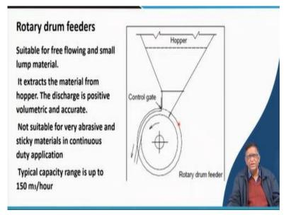
So, these types of feeders are there. Rotary drum feeder as I told you that from the hopper the material is coming out of this, this drum is rotating. The material now which has got flood loaded or contact with the drum, this will be coming and falling it out.
