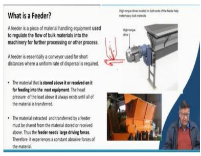
So, there are different types of feeders. Now what is the definition of a feeder? We have earlier also told once again I will tell you about this a feeder is a piece of material handling equipment that will be used for regulating the flow of bulk materials. Now that it is regulating this word is important here because when the material is going it will be just controlling at the time of giving it to the next equipment.
