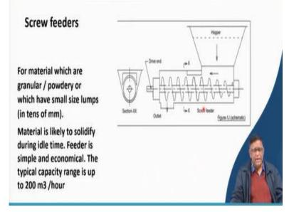
Screw feeder as I was telling a auger type of things will be there, material is coming on to this hopper and then it is rotating and then the material will be going, outlet will be coming through this. So, this type of feeder is a screw type of feeder, this feeder can be used up to 200 meter cube. But if it is a very sticky material, you will not go for it. So, that is a something or many times coal and dry coal can be easily taken over here in the agricultural sector.
