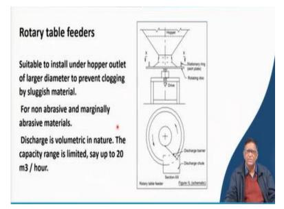
The rotary table feeder you can see from the plan view this is a table which is rotating and there is a discharge the barrier, one barrier plate is there. So, when the hopper material is coming and
