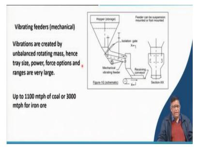
Similarly, in your vibration can be given by a mechanical means without giving an electromagnet, you are giving a making it to vibrate. So, that the whole material which was getting flood loaded over here. From there it is loading on to true distribute to the conveyor belt. (**Refer Slide Time: 34:29**)
