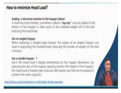
But what happens if you are having a very tall tower silo? From a tower silo that if you are putting over there the whole load if it is taken on the feeder bed to drive it you will have to have a very high torque such a high-power electric motor will be necessary. So, that is why they do sometimes that is your in the inside the hopper they make give some inserts by adding a structural member inside the hopper.
