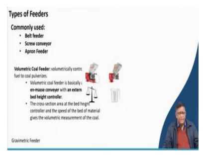
Then there are wide ranges of feeders. But the basic type that means whether you are giving material on volume or you are giving material as a measuring as a weight that is how much. Now why it comes? It is because our bulk material sometimes it could be as a huge quantity when we are talking of the mining and mineral or agriculture sector. There will be agricultural sector will be taking some 100 and 1000 tons of meter cube of material.
