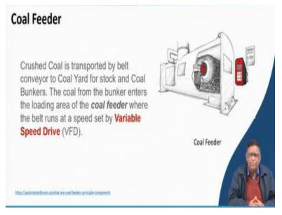
So, let us see few things over here. They apply in a coal this is a coal feeder. What is done here? That is a crust coal is transported by a belt conveyor to a coal yard for stock and coal bunker wherever is there from there it is taken out like that. Now the coal from the bunker enters the loading area of the coal feeder where the belt runs at a speed set by a variable speed drive. Now this is again in the electric motors electric sections you will be knowing about that.
