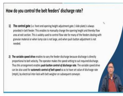
So, how do you control the belt feeder and discharge rate? Now we can control the gate by control gate or a variable speed drive. Control gate means from the bin itself you are allowing the material to flow slowly. That means you will be sensing that conveyor belt speed and how much material over there and accordingly you will opening or controlling the gate. So, that means your digital sensors it will measure this how much material how it is going.
