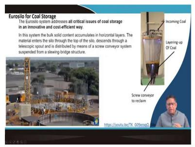
(Video Starts: 07:28) So, you have seen here that this another is when it is a constructed silo, for example, if you that cement concrete silo in a thermal coal, thermal power stations that cold storage, it can get built by step by step that is a huge construction work. That is the civil
