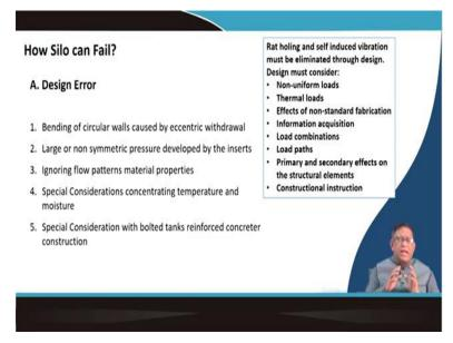
So, when we go for a study of a silo, as they are telling one by one let us discuss that the design error, it can be a bending of the circular walls caused by eccentric withdrawal. That while we are designing the silo, our material should come out that is if it is designed from the center but if you are taking at the that is your eccentrically that means not the center of the of the of your the cylinder.
