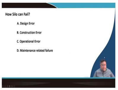
Now, this similarly, we have seen now that there are our reinforced concrete silo or steel silo but there is they are having a lot of potential to fail. Fail means they do not deliver the digit service. And this can be due to design error, due to construction error, due to operational error or due to maintenance related failure. The design error means at the time of designing that whatever the load, it is filled that it will be taking up if it cannot take that load means design, design error.
