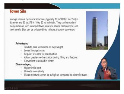
You are not going to that but this silo what we can have the 3 main types that your tower silo your big silo and the silo pile. That were in tower silo, you can see it as a gigantic tower in which the material is spread. Now, normally such type of big tower the material is always fed from the top and by a conveyor belt or other bucket elevator, different types of we will be discussing those bucket elevator and how it can be worked with a silo that for storage purposes.
