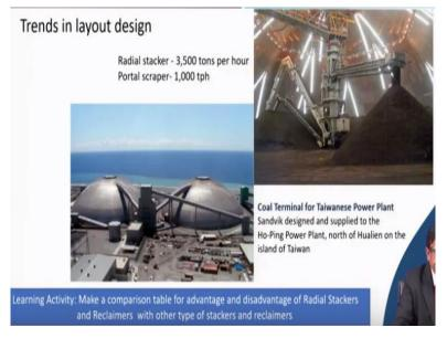
So, there as another thing we have said about the circular stacker. That is your radial stacker. That stacker cum reclaimer it is there. That is a, it can make a circular stockpile. And then, it can collect by a, that is you can see a portal scraper reclaimer is there. As radial stacker is stacking and then this, your, this one is a scraper reclaimer. They are reclaiming the material within a dome. So, this is there are advantage and disadvantage.
