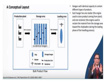
So, that what is the general layout as this figure is showing it in a bulk product flow how it goes. So, that means when a ship comes that is ship to be loaded the materials which may come from the plants from different places by rail or whatever you are bringing from the belt conveyor. So, there could be (()) (14:30) where from your materials are coming and then putting over here. So, then, next thing is you will be having a storage area.
