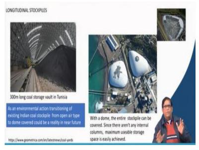
And then giving on the existing while the operations are continuing at that time also, we can have this type of cover for having a better that environmental and better management. In these ones how that company has done for the longitudinal stockpile you can see here along this those stacker and you can now that equipment which you can see here, I think is known to you these equipments your portal or that scraper reclaimer is being used for taking the stockpile out.
