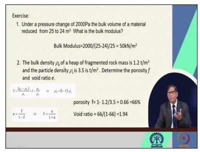
And then you can do a some simple calculations that under a pressure change of 2000 Pascal the bulk volume of a material reduced from 25 to 24 meter cube what will be the what is the bulk modulus? You can find out the calculus the bulk modulus is nothing but
