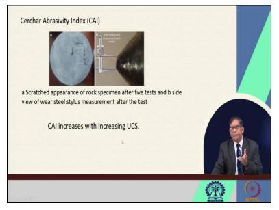
So, you can do also the abrasivity is measured by sensor index you are taking a stylus and that stylus is making say five mark over here after that the stylus has got worn out. Depending on that exactly you can find out that is what is the abrasivity of this particular rock samples such type of things and then researchers abrasivity index it will be if the universal compressive strength of the rock is more there will be more abrasivity. So, such type of relationships are very important.
