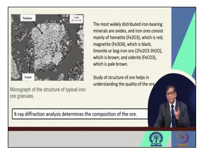
And for that another thing is that the structures of the material in a micro graphs you study and then you find out that how exactly the in a bulk material that where your iron or your other material are present in which form then how they could be liberated in by handling them by processing them. So, these are the things we need to know.
