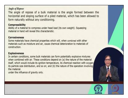
Similarly angle of repose is another very important property if you take a that is a handful of sand and then you start flowing it over there you can find that there is a triangular that a conical step will be formed that means with the horizontal the edge of the heap is making an angle that angle is called your angle of repose. Now this is a very important property while you are making a heap or dump.
