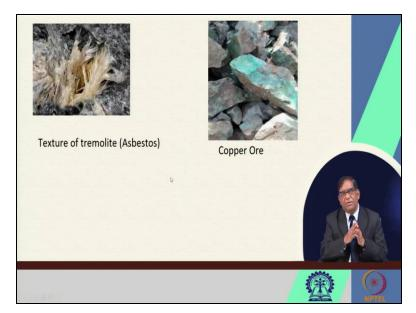
Sometimes some of the materials of course their textures you might have seen that asbestos which has got a fibrous textures or a copper ore you can see the texture with the roughness with the colour that chalcopyrite things which is a bluish nature will be coming. So, many a time the bulk material handling you need to see you can find out whether there are lot of unwanted materials are coming over there or not and then how they will be handled will be depending on those properties.
