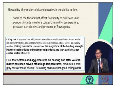
This similarly the granular material how it is doing you will be studying about what is the caking coal or the coking coal in the caking index these are the properties of coal you will have to go through find out these things and they say exactly the caking index is the measure of the magnitude of the binding strength between coal particles and between the coal particles at a particular temperature.
