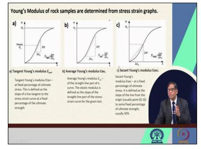
So, similarly for the mechanical properties that Young's modulus that is a very important property of bulk material it can be a tangent young modulus just a stress strain ratio how you can find out that is your when you are putting the stress and then the strain ratio it depending on in which zone you are calculating you can give that average Young's modulus or you can get a second Young's modulus.
