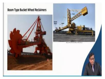
Then the boom type bucket wheel reclaimer, they can be a fixed boom type of bucket wheel reclaimer which can be a rail mounted or it can be crawler mounted. If in a crawler mounted it can move in the stock yard. And then it can, having its discharge boom, which can be positioned over a conveyor belt and they can do it. If you go to naval ignite corporation, they have got number of crawler mounted this bucket wheel reclaimer for collecting the lignite for sending into the thermal power stations.
