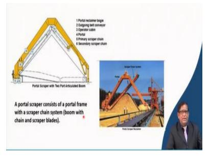
So, there are different systems are there like that you can see here, this is a portal reclaimer. You can see such type of reclaimer this is bringing the material. You can see at the background this is the stacker. And then, once the material is here this side the material is getting collected.
