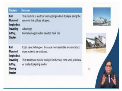
This also we talked about last class. So, here, it can be a rail mounted longitudinal, that means here you are using only the side portions. That means where you are having this conveyor belt the rail mounted stacker it is having a fixed part. Sometimes, if you use a rail that is your crawler mounted instead of having the stacker over here you can just stop it over there. And then, if you can make a flexibility in a movement but there you will have to keep a track.
