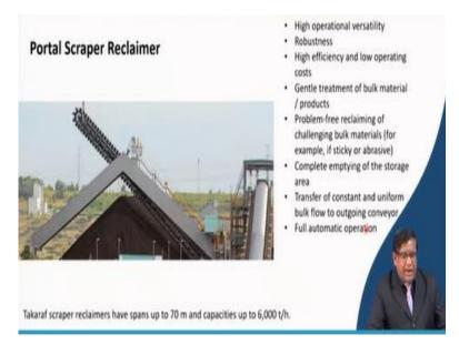
Because of that sometimes they use two scrapers. So, that means here you can see when it is scraping down over here. Only this portion is scraping. But this extra additional length is required. Because when this material will be taking as your stockpiles will get low height. There will be, the length will be, increasing. So, that is why they will be using a double, you can use this side also a scraper.
