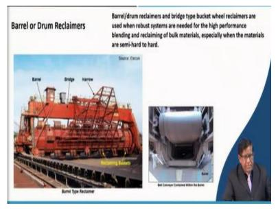
And then there is a barrel type of reclaimer that in which the barrel has got the buckets. Now these buckets will be collecting and inside that there is a conveyor belt. If you see that there a cross section is a circular one in that circular cross sections a conveyor belt is kept so that this bucket which will be dumping the material onto this conveyor belt and they will be taking over here.
