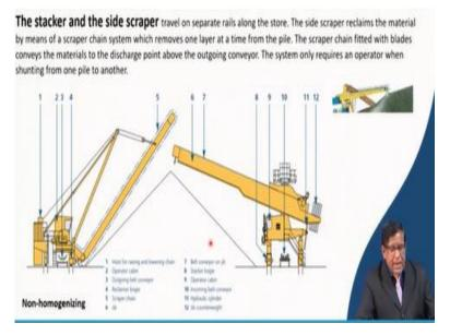
So, if you can see this is a stacker part and this is a reclaimer part. So, these 2 together, they are working for this stock yard. So, here, this that material is being brought over here. From there, with a stacker that arrangement of the tripper that conveyor belt is raised over here and taken into this.
