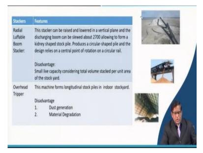
So, that different type of, if it is just an overhead tripper, maybe within a house, if you are to keep your material just free from rain and all there you will have to have an indoor. At that time, your stacking can be just a tripper.
