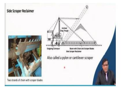
And then, there is another type that is called your scraper reclaimer. In a scraper reclaimer, what is there exactly? You are having a boom or the scraper. Here you can say this type of the scraper that chain, you can see a double chain here, one chain here, one chain here. And then, this is the scraper blade. The scraper blade is mounted. Now, when it will be moving that whole material it will be going and it will scrap over here and it will be loading the charging on to this part.
