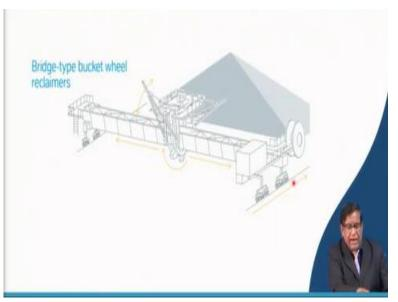
So, in some times, we can have even the bucket wheel ring is there. Now, this is giving a translatory motion over here and the buckets will be in the barrel type, you have seen that
