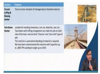
So, you can give the stockpile formed in a different way or we can have a twin boom in which both the sides you can collect it over there.
