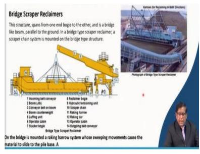
Now this bridge type reclaimer you can see here the components that is incoming material is coming by that. And then this is the boom jib by which they are forming the stock pile. And then here, we have got the conveyor belt on this boom. And there is a counter weight so that it can be balanced over here. And then there will be a luffing unit by which this boom can be raised and lowered. And there will be an operator cabin that operator will be sitting over here.
