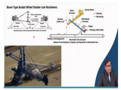
So, that is there, sometimes the same bucket wheel reclaimer can be used as stacker also. So, here you can see the material is coming by that conveyor belt. And then it is coming over here. It is through a hopper; it is and a feeder it is giving to this conveyor belt. And the material is
