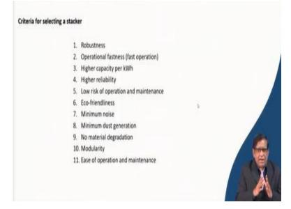
Now, we will be seeing when you were to select in a mines or in your metallurgical plant or in a port particularly in your export terminal where your materials will be coming from different places. And then, you want to do it for the loading on to the ship. At that time, selecting this machine or for that stacker or reclaimer what are the main conditions or the characteristics you will need to look? So, as you said here, the robustness.
