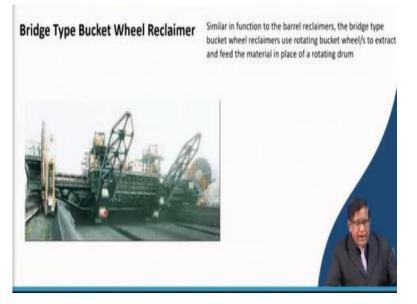
Now that bucket wheel reclaimer, it can have more than one and then say here in this you can see there 2 harrows and 2 bucket wheels are there. And they will be moving collecting the material from this. Both can move in translatory motions here and then the conveyor belt is there in the bridge.
