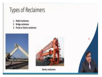
Then your reclaimer, we have said about the stackers that reclaimers can be also of different type. Basically, there are radial reclaimers, bridge reclaimer or portal or gantry type of reclaimer. Now, you can see that this reclaimer is a gantry or a structure gantry means structure. On a structure, your reclaimer is mounted and you are doing it. A portal and gentry they are sometimes used as similarly. But the portal one in which you are having a movable structure.
