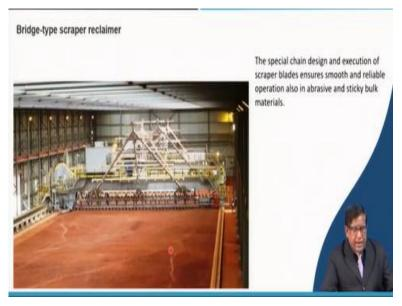
But the other type is a bridge type of reclaimer. In a bridge type of reclaimer, you can see here that this whole reclaimer is forming a bridge. There is a rail here and a rail here. And the conveyor belt is here. Now this is scrapping or there is a chain as you have seen in that scraper, that is there. And it will be taking this whole material and then it will be loading onto this conveyor. Now when there will be a big stockpile here this is the harrow.
