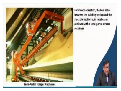
And in this case here so, you can see this. Sometimes, it is a semi portal or hub portal. Inside that, your close type of stock piles, the material is getting stocked over here. So, now, you can see here that how it normally scraps down and then load onto this conveyor.
