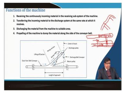
Now that tripper arrangements now, will have to be made into a stacker arrangement you may recall your that conveyor belt basic diagram you know that this conveyor belt it is coming there is a tipper portions over here and that the conveyor belt it goes at the side and then it will be discharging over here to another conveyor. So, that means if you are to form a stacker that is from the conveyor how the material will be brought to the stacker and then it will be taken to the sidewise to dump.
