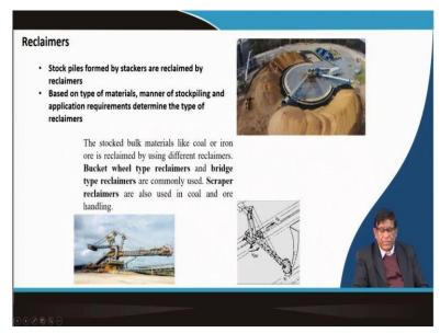
Now, coming to telling about the reclaimers, reclaimer is basically how you will be reclaiming it. If you are forming a circular here and then you start reclaiming from one side and then take the material to the other side. So, it maybe you are collecting it over here and then also reclaiming in a circular pile or this reclaimer can be a bucket wheel type reclaimer from the stockpile. It is collecting the material and sending back to the conveyor belt.
