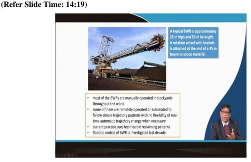
So, you can see here a typical bucket wheel reclaimer. In a bucket fill reclaimer, there will be a will and this will be having its own independent drive and there is a conveyor belt on this boom this is called your cutting boom or receiving boom or that is your reclaiming boom. On that a conveyor belt is there from that conveyor belt the material is transferred to a hopper and from that hopper it comes to that exactly a main conveyor belt which will take the material away.
