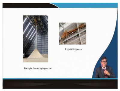
That depends on you are using a typical tripper car here you can see this particular thing here, when you are seeing into this stripper, it is discharging the material and the stockpile is getting formed.
