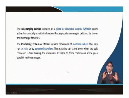
Now, this whole operation when it will take that it can be done by different type of machines. That machines it can be depending on that whether that boom by which the material is discharged it can give a swinging or it can give a laughing up and down depending on that and then how it is moving whether it can move on a rail or it can move on a crawler we can get a different type of stacking machines.
