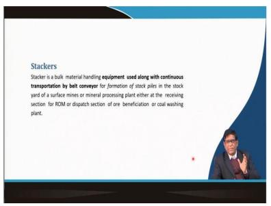
So, these are the different form of stockpile now how what type of equipment will be used for forming this tech stockpile now thing is that depends on how you are carrying the material. If you are bringing the material by a dump truck you just make a heap of material but many a times when you are thinking of getting three million four million ton and then mostly it will be coming by a continuous method.
