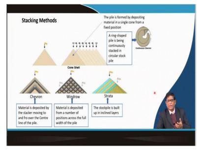
So, this stock piles that to form them there are different type of stock piles. We will be again discussing that why and where this type of stockpiles are used and made. But there all depends on the type of machines by which they are formed. So, that normally a stock is a just a triangular cone and then it will be going on if you put the material, it will be going on increasing by that it is called a chevron type.
