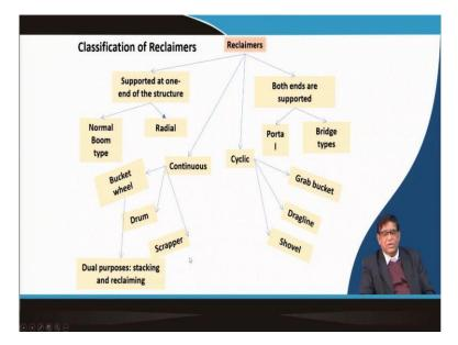
So, now this reclaimer also can be classified by as a supported one and structures or it can be at the both end structures. It can be a continuous type of reclaimer or it can be a cyclic type of reclaimer. It can have normal boom type or it can have a portal type and then there could be a bridge type there are radial type and this continuous can be a bucket wheel type can be a drum type, can be a scraper type, can be grab bucket type, drag line and shovel type of reclaimers are also there.
