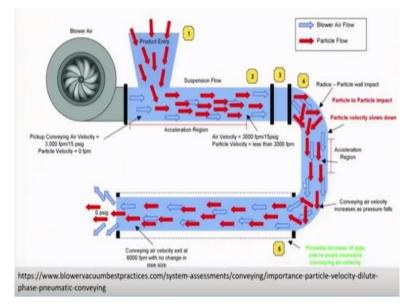
That particles when a blower is going you can see that the particle will be flowing a differently at the bends, they will be striking each other and then it will go. So, now, here, that means at the bend, your diameter may be increased. So, that type of design idea can be taken up by measuring the particle velocities.
