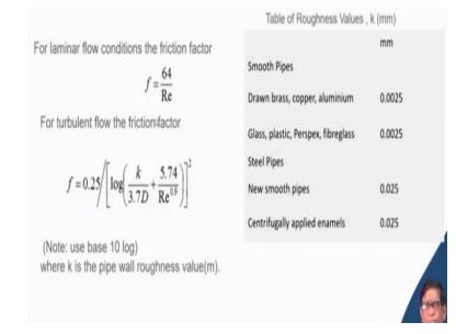
Now, for our laminar flow, that coefficient of frictions can be determined by Reynolds number. And, that coefficient of friction is also can be found out from this equations. This is given in the guide book. That is your the pipe roughness, depending on the pipe roughness that can be value and that pipe roughness which are available in the standard guidelines in terms of millimeter for different types of pipe.
