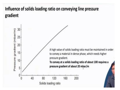
We will have to look into that how density matters. Moreover, another thing is there if your solid ratio solid loading ratio is higher, you will have to maintain a high pressure gradient. When you have to maintain a high pressure gradient that means more energy will have to be introduced into the system. So, that is why you will have to optimize while selecting your system that exactly how much particle and how what concentrations you will be exactly getting.
