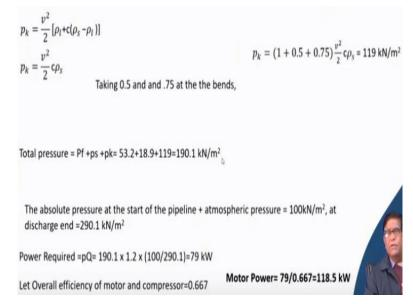
So, by similar way, you calculate all the values. And then, your total pressure some of them will be getting in kilonewton per meter square as given over here. So, this will lead to your what is the absolute pressure at the start of the pipeline. If it is outside atmospheric pressure is equal to your 100 kilonewton then you will have to get this much pressure exactly (()) (31:31) introduced into the system. At the delivery end, your pressure will be then 290.1 kilonewton.
