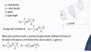
Then that another thing is their pressure due to the sliding friction of the solids. Now, when the solid will be touching over here, at that time, this solid force that also that is the frictional force also will have to be taken out. Now, it will depend on that mass flow rate of the solid. That is your total tolerance. That is how much tonne per hour it is going. On that basis, will be calculating it out.
