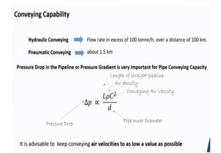
And then, they determine. Now, what you exactly do that experimentation. It is for the your in case of hydraulic conveying, the flow rate you can get at about say excess of 100 tonne per hour for a distance of 100 kilometer it can go. But, in case of your pneumatic conveying, as I said, it is a, for very less distance because that pressure gradient in a pipe conveying follow this one. So, that means you can see that this velocity is squared.
