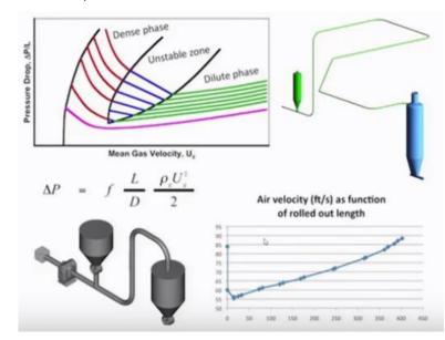
So, one thing is there that pressure drop which we can we are measuring by D'Arcy's formula, it will be depending on the type of flow. In a dilute phase, it will be working over here in an unstable zone and also in the dense zone. And, as your loading factor is increased,
