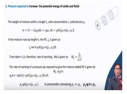
So, this is the way how you do also for increasing the potential energy of the solid and fluid. Now, that whole solid and fluid is moving from one point to another point. At that time, the total pressure required can be calculated by and from there you can find out this pressure. For, that is your what will be coming for the increasing the potential energy.
