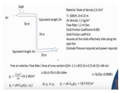
Now, you can take up a small problem. Say, for example, your air is introduced over here. Compressed air may be pressurized or by vacuum creation positive or negative pipeline you can take it over there. Solid is introduced here. Let us say 50 meter it has gone. Then, there was a bend and then which can be considered as an equivalent length of 2 meter. Then, you have got a path for 70 meter. Then, you have got another part for 20 meter.
