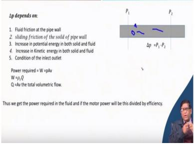
So, if you just think of there that in a pipe at a 2 separated distance. Here, the pressure is P 1, air pressure, the P 2. That means a pressure drop has taken place over there. And, it will be depending on that number of factors. First 4 factors are very important. That is fluid friction at the pipe wall. When this fluid will be flowing through this, at that time, they will be giving a, exactly here the flowing fluid.
