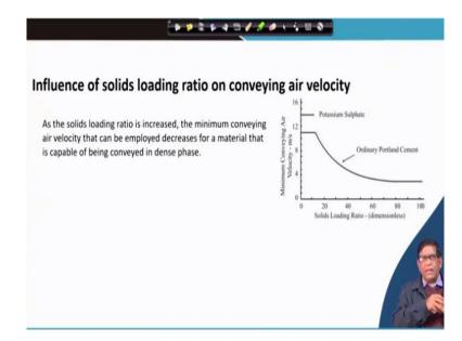
Now, that your solid loading ratio it exactly plays a very important role in pneumatic conveying. Exactly as the, that your loading ratio is increased, the minimum conveying air velocity it gets decreased. You can see here. That is, your, the main velocity here is less but that your solid ratio is coming more. That means if you want to increase your solid ratio and then you want to increase the, this velocity also, it will be giving certain problems.
