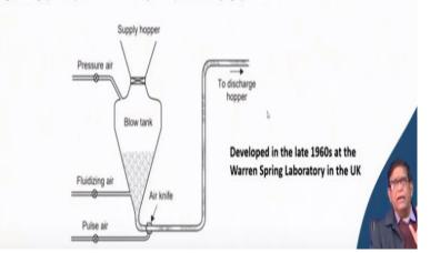
But, if we want to get how to transport fine materials of a cohesiveness or that are difficult to convey. You can find here a fluidized air is given, pressure air is given and also a pulsating air so that this will be giving making them to flow as a plugs. It will be flowing over here. So, like that many different types of systems can be there.
