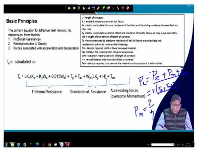
Now, let us see over here that you are having this primary tension the T e it is coming off as I said that the frictional resistances then resistances due to gravity and forces associated with the acceleration and decelerations where the resistance is coming from the belt getting that sort of bending and then over the rulers then there is a frictions all these things coming over here.
