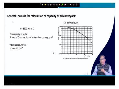
Then, one thing is there you have now learned that how to calculate the area of cross sections of the material, you have seen also how you get the belt width. Now, once we know the belt width and once we know what is the cross sectional area of the material, you can find out the capacity. If it is for all conveying systems your capacity is given by this in ton per hour that is your rho is the density.
