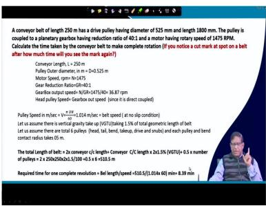
Now, for this let us go for a very simple calculations here. A conveyor belt of length 250 meter has a drive pulley having diameter of 525 millimeter and length 1800 millimeter the pulley is coupled to a planetary gearbox having reduction ratio of 40:1 and the Motor having rotary speed of 1475 rpm. Calculate the time taken by the conveyor belt to make a complete rotation.
