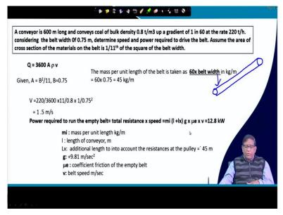
Another problem you can check over here that is a conveyor is 600 meter long and conveys coal of bulk density 0.8 ton per meter cube up a gradient 1 in 60 at the rate of 220 ton per
