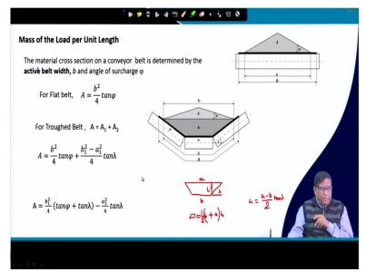
So, next, the sizing is your how much will be the mass of the load per unit length. So that means, your the sized material or un–sized material is there then in your one meter length. How much material will be there? That is another things that in a flat belt, you can see over there that in the belt. You will have to have both and some of this you are free and will have to be there.
