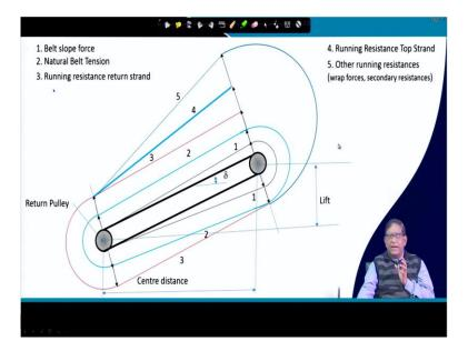
Now, how you calculate that? Suppose this is a conveyor belt. Here, 2 things will be there, this belt when it is running over these 2 pulleys and then carrying the material upward, there will be this belt must be under tension. So, there will be a belt force and natural belt tensions we will be working over there. Then what will be there? There will be another force that is your with the help of the there is a return pulley.
