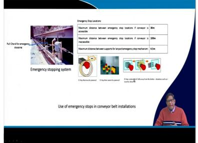
Now there is a pull chord switch which is exactly all along the conveyor a chord is there and there is a switch now this switch is through relay and contacts connected to the main drive motor circuit this pull chord circuit is connected through relay and contacts. Now if you press there and these are this pull type of button if you just pull it anywhere. Then it will trip the motor power supply to the drive motor will be obstructed.
