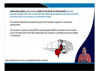
So exactly a proper running or proper maintenance of a belt, we should not have more creep or slip then what is there exactly they say we can monitor this creep or slip by knowing exactly what is the relative motion between the belt and the drum. And then for that, we need to get this pitch switches. What they do, if your both the you are driven pulley and driving pulley, if they are running at the same RPM, then we assure that there is no slip of the belt.
