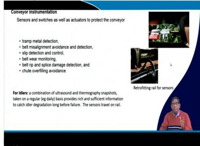
Now, today, there is a lot of that people are trying to do start up for developing new instruments and then so that the operations of the conveyor belt can be improved. Nowadays the different types of sensors and switches are there the tramp metal detections, this is another
