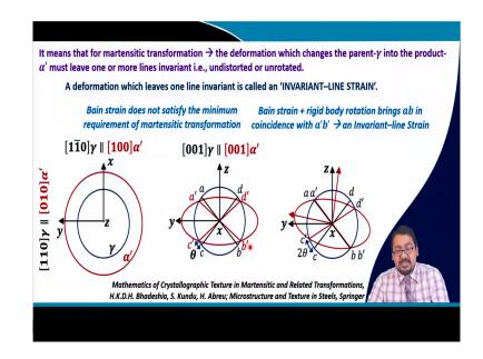
So, it means that during the martensitic transformation, the deformation which changes the parent gamma austenite into the product alpha prime martensite must leave at least one-line invariant, which allows the line vector of the dislocation to move through it through the interface from the parent to the product phase without any distortion or any rotation. A deformation which leaves one-line invariant is called an invariant line strain.
