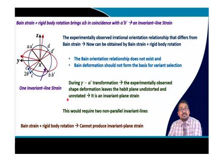
So, what I am saying is that that with a rigid body rotation along with the Bain strain can bring a, b in coincidence with a prime b prime therefore, it becomes an invariant line strain. So, the experimentally observed you know the martensitic transformation if you observe experimentally, it contains an irrational orientation relationship that differs from the Bain strain.
