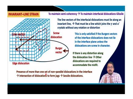
So, what is the importance of invariant line strain here? In order to maintain the semi coherency that is to maintain the interfacial dislocation glissile, the line vector you see if we are looking into this structure which shows an edge dislocation here right, and the screw dislocation here, we all know that our dislocation is actually a loop which contains a screw dislocation somewhere here, an edge dislocation somewhere here.
