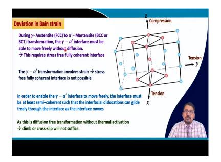
So, now we have as we have learned in the previous lecture the Bain strain, we have seen that there is a negative strain in the z direction and positive strain in the x and the y direction of the BCC or BCT martensite which is forming. So, while this transformation takes place from the gamma austenite to alpha prime martensite, the interface between the gamma austenite and the alpha prime martensite should be such that it should be able to move freely without any diffusion processes occurring.
