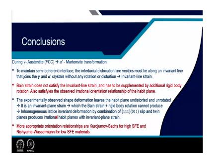
So, in this lecture class, we found out that during austenite which is an face centered cubic material to alpha prime which is martensite and is a body centered tetragonal or body centered cubic material transformation. In order to maintain a semi coherent interface the interfacial dislocation line vector must lie along an invariant line that joins the gamma austenite to alpha prime crystal without any distortion or any rotation.
