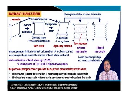
And so, if we look into the invariant plane strain scenario let us take an austenite which looks like this a gamma austenite and if we introduce an invariant plane strain to this. The observed shape change during the process is correct, but the crystal structure that is obtained is different from that of the alpha prime martensite.
