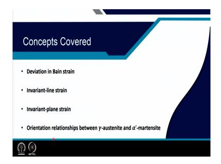
So, the concepts that will be covered in this lecture is deviation in Bain strain. We learned Bain strain in the previous lecture and then what is invariant line strain and invariant plane strain, why it is necessary to have an line invariant or a plane invariant during phase transformation. Then the fourth one is orientation relationship between gamma austenite and alpha prime martensite other than the Bain transformations that we know.
