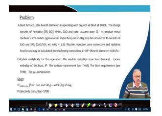
So, now, Now, consider the problem given in the slide above. <u>some problem that is a</u> problem is a<u>The</u> blast furnace is operating with the dry hot air blast at 1400 Kelvin. The charge consist of hematite, sinters, CaO, <u>and coke</u>. Its product metal contain 5 percent carbon, and its slag <u>maybe consider consists</u> of CaO and SiO<sub>2</sub> at a ratio of 1.2. , all these
