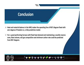
**So**, in conclusion we can say that because of the presence of a well defined thermal and chemical reserve zone in blast furnace, it is conceptually possible to divide the blast furnace into two zones and make heat and material balance separately.
