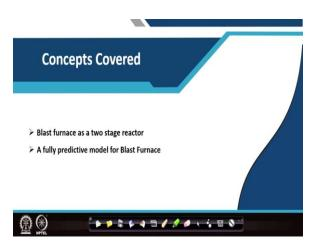
The basic concept covered are: blast furnace as a two stage reactor; this is a very important concept and we have to understand that blast furnace can be conceived as a two stage reactor. And then we will develop a fully predictive model for the blast furnace where the operating line will be fixed by developing two fixed point on the operating line. So, optimum and the minimum coke rate can be predicted for a fixed charge in Blast Furnace.
