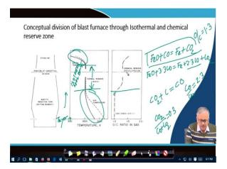
Now, we will discuss the conceptual division of the blast furnace through isothermal and chemical reserve zone. Now, let us see the temperature profile of gas and solid, the second diagram from the left. Here, solid line represents the axial temperature profile of the solid above the tuyer line and the dotted line represents that of the gas.
