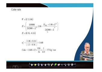
So, then wustite reserve zone you have this point, there is a thermal pinch point, you have the this is the chemical pinch point is known its constant 1.3, 1.06, because basically this is the wustite equilibrium composition. And then the thermal pinch point is given like this.
