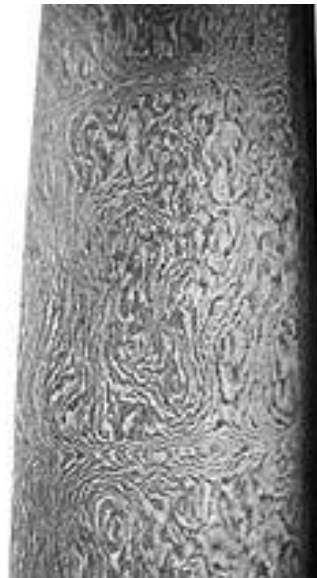
Figure 26.2: Wood grain microstructure of Damascus sword
