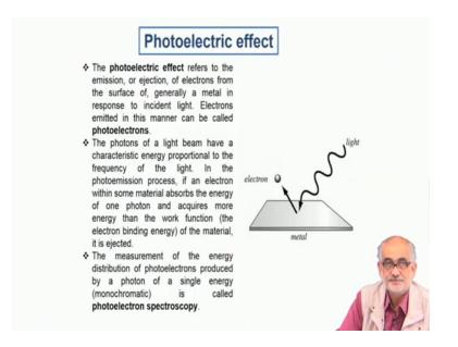
Electrons can be emitted also because of excitation coming from optical ray in some metals we if we have or particularly on some because of certain coatings we actually can see a situation, where incident wavelength can raise electrons from the valance to conduction band.
