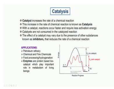
So, catalysis is another such phenomenon I mean its very simple to for us to understand the way the catalysis works that if you actually imagine a hump like this such a big hump. So, it actually shows that you have a large barrier to cross. So, instead of this big hill if you have smaller helix to actually cross which is going to be much easier and that is exactly what happens when you do catalysis.
