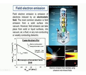
So, thermionic emission is a phenomenon or a property which is dependent upon the ability to emit electrons from the surface due to excitation purely which is of thermal in nature. We can also have field emission phenomenon where electrons are emitted because of the application of field electrical field and such kind of phenomenon is utilized in for example, this scanning electron or transmission electron microscope where we have this large column.
