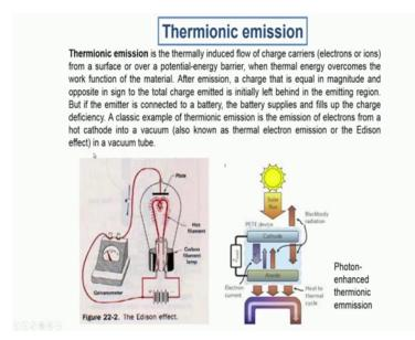
Um So, until now the entire effect was due to the reaction to an excitation coming from optical rays and instead of emitting light we actually can even emit electrons and this emission can happen because of multiple possibilities of excitation. Over here when we talk of thermionic emission we are talking about a situation where we apply a very high amount of potential difference and current.
