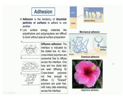
When we need to actually glue two different surfaces, two different dissimilar surfaces the adherence of these two different surfaces visually which will largely depend upon the adhesive forces that we can create either by either by themselves. The two surfaces can have a natural tendencies of aeration or we can apply material in between for example or a clue or a gum which actually can lead to chemical adhesion.
