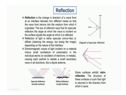
For various purpose for example, the surface of a mirror you would not like to have a situation which is like this. If you have a lot of roughness on to the surface then the incident beam will get scattered in all directions and then the reflected light will have certainly not be able to gather all the scattered rays and not only the image could be distorted, but more importantly the intensity of the image that you will create will be weaker or poor.
