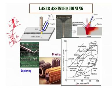
Another very major application is joining. Now, joining not only of similar type where. So, there are 3 possibilities actually one can think of, if we want to join a solid body A and B together, we can simply heat here, such a way that this part melts and some part of the beam melts and eventually they fuse with each other. So, it is a fusion joint created by partial melting of A and B at the edges.
