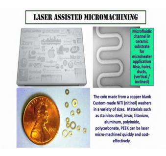
That can be done very easily on laser on metallic surface. So, here is an example from a commercial house that you can create so many markings. So, many types of marking can
