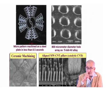
So, the same micromachining patterns could be done on steel, on semiconductors, on polymers, on any solids and with very large aspect ratio the like this nano pillars of carbon nanotube or you can drill holes on a silicon wafer, maybe a few almost half a millimeter or so deep or you can create channels and vias and various other structures of very specific dimension.
