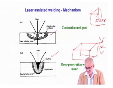
For joining, we already discussed while discussing electron beam assisted joining that if. So, here is the importance of locating or the location of the. So, if this is the solid we are talking about and so, we have 3 possibilities, we have the possibility of the focus, resting above the surface, we have the possibility of the focus, coinciding with the surface or the focus going below the surface.
