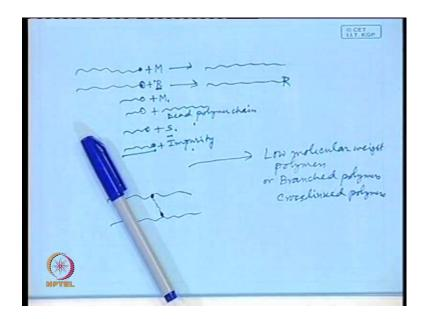
The chain is growing when it is supposed to add to monomer giving bigger chains, but it interacts with R radical. So, it can stop over here that is a transfer. That means this activity is transferred to this primary radical. Now, this activity can be transferred to a monomer. Not only that, this activity can be transferred to a polymer chain, a dead polymer chain, this activity can be transferred to a solvent, so the present monomer, dead polymer chain, solvent and some impurity.
