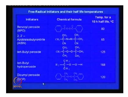
This same thing in another way it is shown effect of initiation radical initiators and their half life temperatures. Half life temperatures are given over here. The formulas are shown over here and half life temperatures are shown. You can see in the net. That is all.
