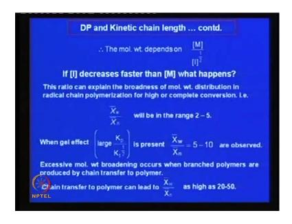
Now, here let us consider one parameter. You have been acquainted with a parameter number is degree of polymerization. You can have another parameter weight array degree of what is number of arrays, what is weight of arrays. (Refer Slide Time: 20:45)
