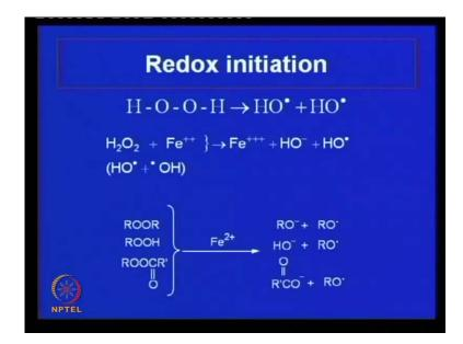
Redox initiation what is redox initiation? That redox initiation is more advantageous than thermal initiation because redox initiation can be carried out at very lower temperature lower than ambient temperature. Even say if you take hydrogen peroxide and ferrous system ferrous salt and hydrogen peroxide that produce on as well as free radical.
