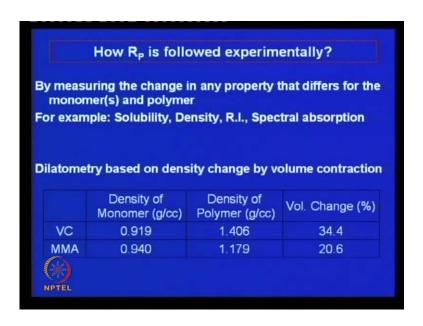
Now, the question is how this rate of this polymerization is experimentally followed how it is evaluated well. You can say sir, you are showing us with the help of these expressions or equations that this is the way to get this rate of polymerization, but how to experimentally evaluated. Suppose you are given this assignment of synthesizing poly
