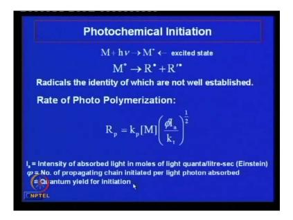
Photochemical initiation monomer the monomer and this is the light h v and this is the excited state of the monomer, when it absorbs the light of a suitable wave length. Now, this once this monomer is excited by light the disassociation the bond of that monomer by bond that disassociates producing free radical, R dot and R prime dot and that initiates polymerization. Now, there are other considerations too.
