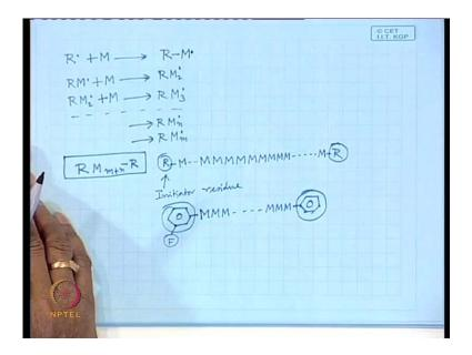
You have seen in case of thermal initiation that sequences of events, that you have seen that primary radical R that adds to the monomer at the initiation step for being an
