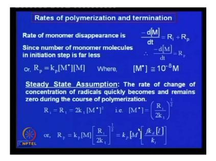
So, what will be the rate of polymerization, now the rate of polymerization depends on this monomer disappearance. So, the monomer disappearance rate is expressed as minus d M d t where M is concentration term that is the sum of two rates, rate of initiation of monomers as well as the rate of propagation you have seen the propagation steps.
