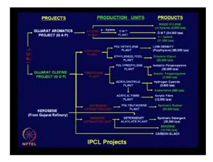
When we say in 1970's actually in 1970's, the first petrochemical complex was set by Indian petrochemical corporation of India at Madhudara, for manufacture of or cracking of naphtha, the refining of crude oil. Then cracking of naphtha, by cracking process different types of organic chemicals were manufactured. So, it gives a close view of different projects taking up by the IPCL that time and here you see different chemical compounds xylene, then polyethylene and these are the a polymers.
