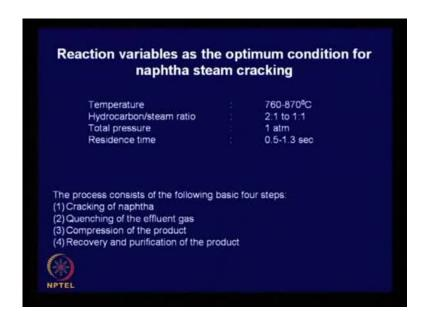
Reaction variables as the optimum condition for naphtha steam cracking, this steam cracking. There was I already shown to you, and look at the reactions came in catalytic cracking.
