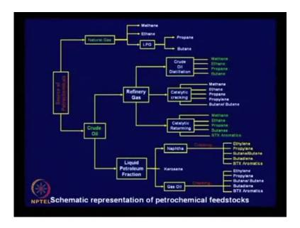
This source is schematic representation of petrochemical feedstock's. These are the varies petrochemicals here you see, we are mentioned here methane, ethane, propane, butane, propylene, butane, butane, btx, benzene, toluene, xylene, aerobatics etcetera. So, these are obtained from either crude oil or natural gas. These are praxinated from this we get LPG, liquefied petroleum gas, cooking gas. This contains propane propane and butane and from
