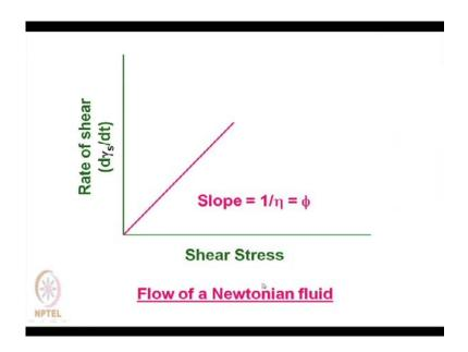
And, if we make a plot of rate of shear stress rate of shear rate of shear d gamma s dt rate of shear is rate of shear d gamma s dt deformation rate, rate of deformation we can say and this is shear stress. So, shear strain rate, we can also say shear strain rate versus shear stress card, these also linear in case of a non Newtonian fluid, a Newtonian fluid. So, we see the, we see that, this is the a Newtonian fluid or an ideal fluid.
