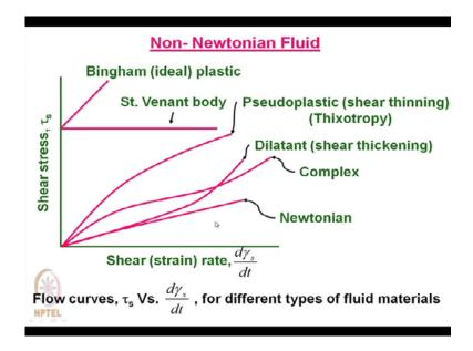
Now, our polymer materials are Nonnewtonian materials or non Newtonian fluid. So, the peculiar behaviour where, now here if we make plot of shear stress versus shear strain
