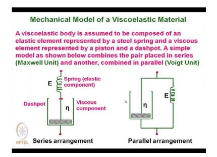
And that viscoelastic phenomena can be explained with the help of mechanical products one is Maxwell model and another wire model. This is the Maxwell model where, that
