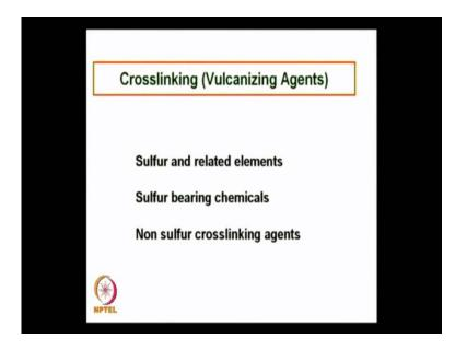
These are not new cross linking vulcanizing agents assignments and sulfur and related elements. Sulfur bearing chemicals non sulfur cross linking agents these are vulcanizing agents used for making a rubber products.
