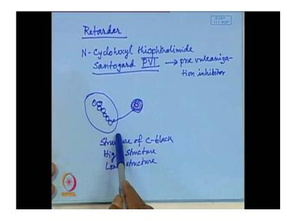
So, 1 nodular can consider like this. They are such they are inside the layers are there. 5 layers are there. So this is these are fused together. So here is the fusion here is the fusion here is the fusion. This entire fusion fused nodular structure is known as structure of carbon black. There are high structure carbon black and low structure of carbon black. High structure means high extent of nodular fusion low structure means lower structure lower structure extent of nodular fusion.
