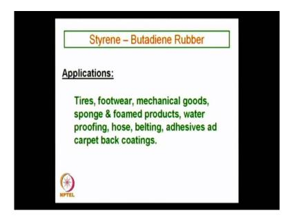
Styrene butadiene rubber applications tires footwear mechanical goods sponge and foamed items, water proofing items, hose belting, adhesives carpet back coatings. Sometimes see lands, sometimes rubber coated fabrics and, so many that means large number of products can be fabricated from synthetic rubbers. As well as from natural rubber.
