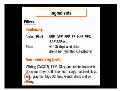
Now come to the details of the ingredients look at the fillers. There are two categories of fillers Reinforcing fillers and non-reinforcing fillers in reinforcing fillers. That increases the improves the strength properties of the rubber compound by the presents. That means they enter in to a direct interaction between the polymer and the filler. There will be if there will interaction polymer and the filler then we call it is a reinforcing filler.
