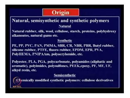
This polycarbonate is a polymer, it is a transparent polymer, color less transparent polymer or you can make it colored also. It is strong; it is rest into delivery temperature, so these are used for making baby feeding bottles, which can be sterilized, polyamides different types of nylons are possible. As you are seen here polyamides nylons or nylons can be both aliphatic and aromatic depending on what reactance you have selected.
