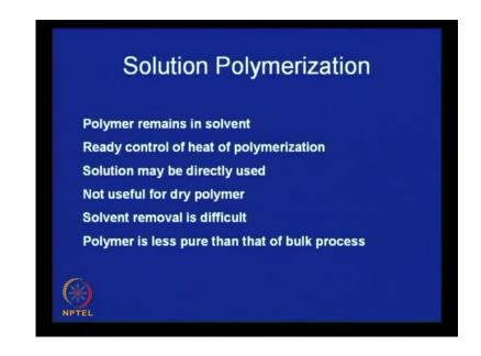
Next, let us see polymerization in homogenous system. So, you have seen bulk polymerization. Some installations where different units are involved for getting a polymer granules or flakes or fibers etcetera from a homogenous system and you have seen the merits and demerits of their bulk polymerization. In a heterogeneous polymerization system or a homogenous polymer sorry here will come heterogeneous polymerization system later.
