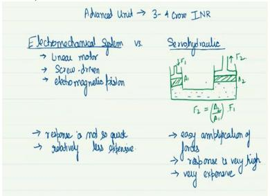
One is the electro mechanical system versus servo hydraulic. So in this one you have basically a motor so something it may be a linear motor which causes. The movement up and down movement of the sample of the cross head, or it can be a screw driven system. So it is a motor, which rotates the screw and because of which the cross head moves up and down. Or it can be electromechanical system, which pushes the Piston up and down electromagnetic system.
