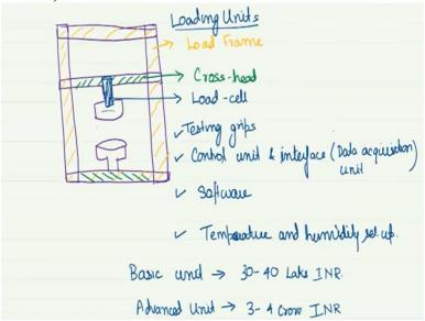
So let me draw simple schematic of how a UTM looks like. So, there is a frame now it is supposed to be vertical although my drawing may not show it exactly like that. So, this is a frame and this is called a double vertical frame. There can also be a single vertical rod for supporting it and it all basically determines what will be the total cost of the equipment and in here you would have a testing job somewhere over here.
