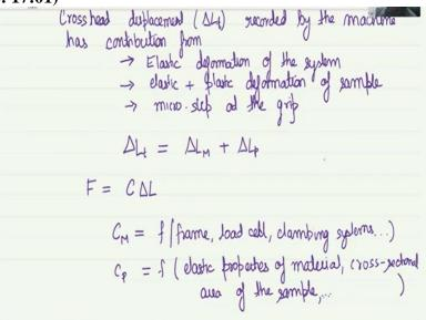
Let us look at what is the relation between  $\Delta L_t$  and the  $\Delta L_M$ , which is the displacement of the machine plus  $\Delta L_p$ , which is the displacement of the system. Now we know that force is equal to. What is? Where, is the stiffness so if stiffness is the C times,  $\Delta L$ . Now, stiffness for the, what is the stiffness of the machine, and its stiffness of the Machine, this is related to the frame.
