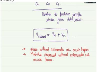
So the V deformation or the V cross head =  $V_M$ . So, the rate at which the machine is deforming plus the rate at which the sample is defined. So these 2 things together, clearly tell us that the data that we obtained from the equipment has to be looked at carefully understood properly. And if you do not carefully, partition the data you may get very erroneous data. For example what you would observe is that?
