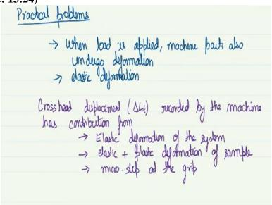
The Practical problems that can arise in a machine and because of which so much science and engineering goes into making this machine is that. When you are applying the load, you should also realize that it is load is also being applied back onto the equipment and therefore the equipment will also deformed. So first let me write when load is applied machine parts also undergo deformation. So what type of deformation would it be?
