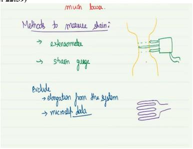
Whenever you are trying to get good quality data used for which you can use the publication then you have to measure strain using one of these techniques. In fact, some of the papers and reviewers will not accept the data if it has been, if where the Strain has been calculated directly from extensometer. So, one of the methods is extensometer. So extensometer is basically showing device which sticks onto the surface of the sample.
