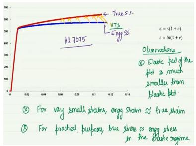
So the equation is given over here so sigma is the true stress and s is the engineering stress so it is given by related to each other by (1 + e) where e is the engineering strain. And epsilon is equal to epsilon which is the true strain is related to the engineering strain by epsilon = ln(1 + e). Now let us look at this data this has been obtained by a professor in his lab for aluminum 7075
