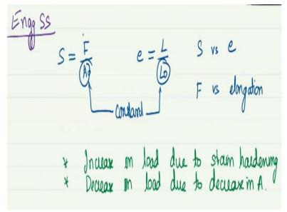
So here stress is given by  $S = F/A_{\circ}$  and strain is given by  $e = l/l_{\circ}$ . Now you see that what is  $A_{\circ}$  it is the initial area at the beginning of the test similarly  $l_{\circ}$  is what it is the initial length at the very beginning of the test. Now when you keep doing the deformation this quantity and this quantity is not changing. They are constant so in affect S versus e depicts nothing but force versus elongation.
