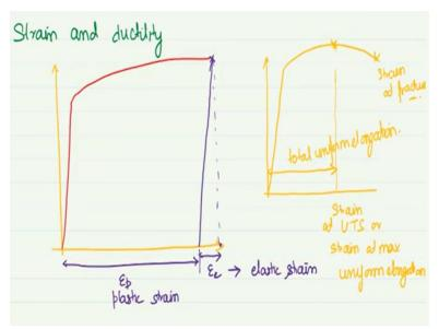
So we have already looked at strain at great length but now we will also look at some more parameters related to strain. For example there is uniform along uniform strain there is strain up to fracture these are 2 other parameters then there is plastic strain there is elastic strain. So again let me so let us say we are at the point UTS so if we drop the load then it will come down and it will follow the slope almost that you have in the beginning.
