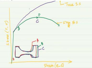
And therefore we need to understand what is the difference between these 2 and let me just correct this part. So now it is true stress strain versus engineering stress strain so we need to understand what is true stress strain and engineering stress strain. To being with again you may have seen the plot for true stress strain versus the engineering stress strain and this is how it will look like the schematic I am drawing a schematic.
