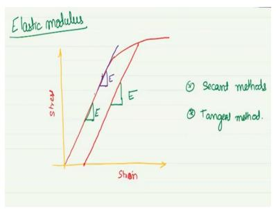
So we have already seen the origin of the elastic modulus and in today in this part we will look at how to calculate the elastic modulus from the stress strain data? But to warn you that the data that you obtain from stress strain is not very accurate for measuring elastic modulus, and it is rarely done and really you use the stress strain data to calculate the elastic modulus of a material. But nevertheless since you have data you can use it to obtain elastic modulus.
