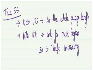
On the other hand when we are talking about true stress strain curve depicts up to the UTS it is depicting for the whole gage length because the deformation is taking place in that whole volume. So coming back to this diagram so up to if you look at A and B under C up to A B and just before C. C is actually some uh to be more accurate it is somewhere which is beyond P just beyond point P.
