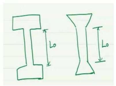
On the other hand one of you is other friend test a sample which tests like this sorry which looks like this. So very orthogonal in shape on the other hand still another friend test the sample which is trapezoidal heads. On the other hand you have tested a sample which looks like this so the question is would you get the same stress strain behaviour for all of these?
