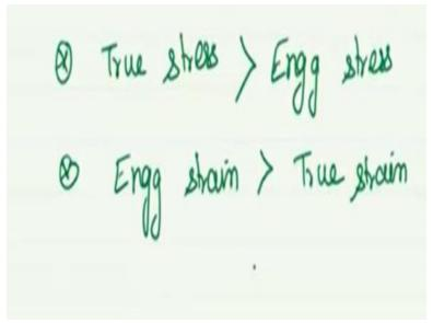
Another point to note is that if you go by this equation then you would note that the true stress is always higher than engineering stress. And the other aspect is that engineering strain is always greater than true strain. The implication of this is that you would always see the curve that equivalent points would always be like this. So it will always be the in true stress strain curve would always lie to the top left top hand left of the engineering stress strain curve.
