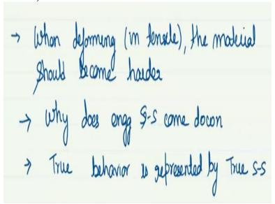
Now we know that when you are deforming a material or basically stress strain is also deformation so when you are deforming the material in tensile the material should become harder right. So this much is clear then the question is if the material is becoming harder meaning you need to apply higher stress then why does the engineering stress strain come down.
