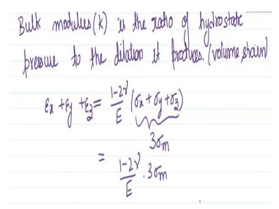
It is the ratio of hydrostatic pressure we are not yet gone into the details of hydrostatic what is the hydrostatic and what is deviatoric? For now just we will define and then we will come back and revisit what is hydrostatic? So hydrostatic pressure to the dilation it produces dilation meaning volume strain. So volume strain is what basically  $\varepsilon_x + \varepsilon_y + \varepsilon_z$ . Now if you look at the above relation then you can add these and what you will get is this
