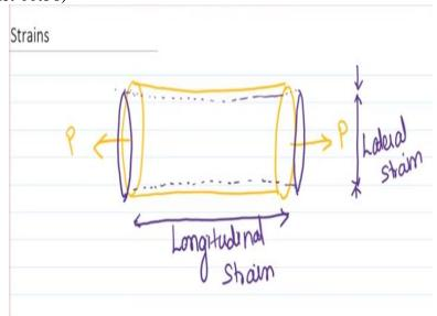
So if you have a cylinder let us say and you apply a force on it and pull it out then the cylinder gets elongated and in the process there is some strain. So how does the strain look like so let me draw it here it is not difficult to draw. So let us say this is a cylinder and although it looks like it is not parallel but the sides are parallel and then you are applying some force which will convert to stress.
