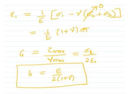
And therefore this is  $\frac{1}{E}(1+\nu)\sigma_1$ . Now for getting the relation for the shear modulus we know that shear modulus is equal to  $\tau_{max}/\gamma_{max}$ . But what is  $\gamma_{max}$ ?  $\gamma_{max}$  is nothing but 2 times epsilon 1 and  $\tau_{max}$  is nothing but  $\sigma_1$ . So whatever relation we have derived is for the condition of pure shear but then if it is the relation between G, E and  $\nu$  then it must be valid for all conditions.
