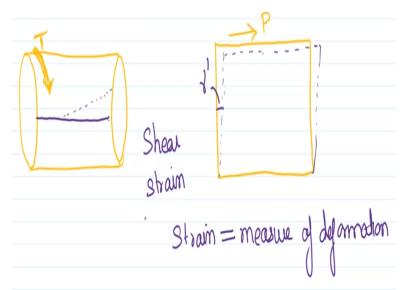
So let us draw again the cylinder so the torque is being applied so this is a torque and the strain is also this is the plane of the torque and the strain is also in this plane and therefore it may look like this so what it is showing is that originally the line may have been like this. But now that you have twisted it like this so this line may appear bent like this and if you open it up if it were a hollow cylinder then how would it look like.
