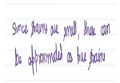
So since strains we are assuming that or the other way down we are assuming that the strains are small. So we can take them to be equal to true strains so moving on now we will have seen the formal definition of strings now let us look at strain as a tensor quantity.
