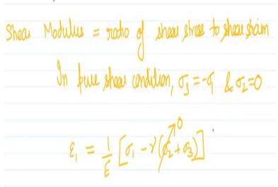
So shear modulus so this is the ratio of shear stress to shear strain to get to the equation for this what we will do is? We will go to the pure shear condition in pure condition sigma 3 = -sigma 1 and sigma 2 = 0. Now if you write sigma 3 = -(sigma 1) then we can go to this relation and put the value over here. So again like I said that here what you are doing is you can instead of epsilon x; you can say it is
