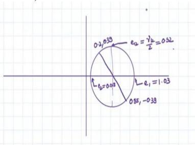
So we here is our circle just shift it a little bit here now let me zoom it a little bit. And one particular condition is known to us so the values are like this so we have calculated f strain x 0.85 strain y 0.2 and epsilon x y 0.39. So one of the x plane x y will be 0.39 and other will be -0.39 so the minus we have the way we have drawn here is in the higher side of x normal stress normal strain.
