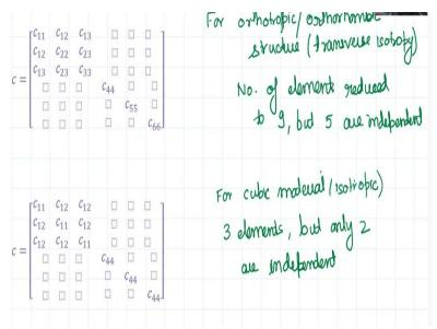
So your independent quantity is so this can be reduced to so basically let me be more specific based on symmetry. Sorry this is not symmetry based on equivalence of value this matrix can be reduced to 21 elements earlier we had 36 elements. However we are not satisfied with this one because we know that there are something some more conditions that we can apply and hence we can reduce it.
