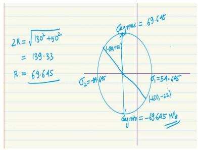
So if have to draw the Mohr circle for this how would it look like so one of them is negative minus a t and one of them is positive and there is also shear stress if it is here then it should also be here. And therefore both of them have shear stresses acting and therefore none of them are principle stresses. So the principle stress values would be higher than these. Now let us draw it and the condition what that we have here based on that we can say?
