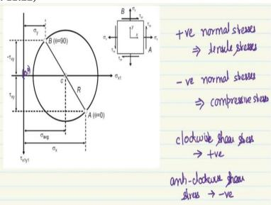
So let me copy image which will help us understand better so here is our Mohr circle. Like we mentioned on the x axis you have the normal stress and on the y axis you have the shear stress. Now for the Mohr circle normal stresses which are positive in values so positive normal stresses imply tensile stresses. And the negative normal stresses imply compressive stresses. So that is one important aspect when you are looking at the Mohr circle and in that respect.
