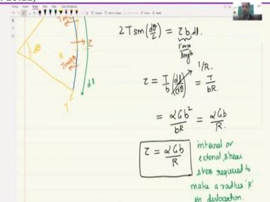
And therefore, this relation translates to T/bR. And T we know is nothing but the  $\alpha Gb^2$ . Therefore this becomes  $\alpha Gb^2/bR$  which is equal to  $\alpha Gb/R$ . Therefore, you need a shear stress equal to  $\alpha Gb/R$  with this can be internal or external, internal or external shear stress required to make a radius R in this location.
