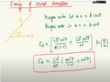
So let us say you have a dislocation going like this so that we are looking at a segment, which is straight and therefore the line vector is like this, but the Burger vector is given like this so that this angle is theta, which means that the Burger vector component parallel to u is equal to  $b \cos \theta$  and the Burgers vector perpendicular to u is equal to  $b \sin \theta$ .
