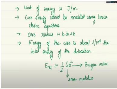
So couple of things are important to note here that the unit of this energy is joule per meter because it is energy per unit length. Another thing that we have already emphasized is that core energy cannot be modeled using linear elastic equations. We have already seen that the core radius is usually taken from b to 4b. It depends upon the model on the researcher.
