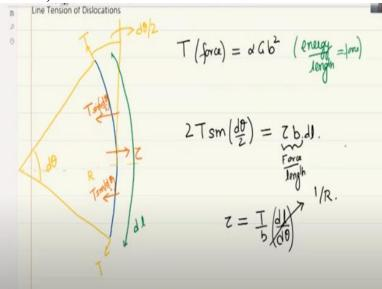
So let us say that this is a dislocation which has been curved because of some shear stress. So now, I will show the shear stress like this. Shear stress is acting like this  $\tau$  and there is also line tension, okay. So the line tension will be acting along the line direction at that particular point. So this is assuming a very small region and so we will assume that this is a very small segment which is  $d\theta$ .
