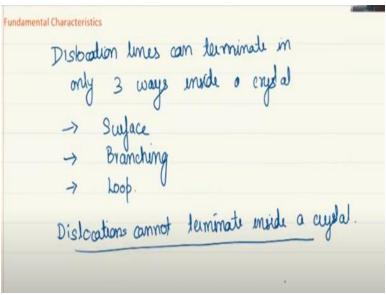
The three ways are one, the dislocation, end of a dislocation command can come onto the surface. And therefore it will create a step and with that step it will get terminated. So it can get terminated on a surface. That is one way for a dislocation to terminate. Another is by branching. So let us say one dislocation, it gets branched out into two other dislocations.
