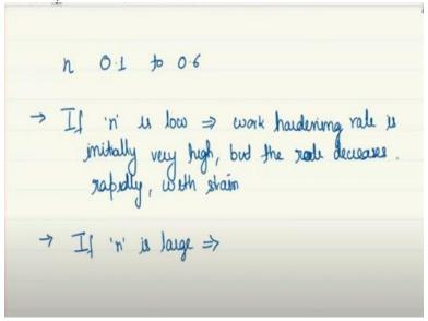
So we see that n can have a range of usually of the range of 0.1 to 0.6. If n is low, then what it means that the work hardening rate is initially high, but the rate decreases very rapidly, I will schematically draw to explain it, but the rate decreases rapidly with strain. On the other hand, if you have n as very large, relatively large, then it implies that work hardening rate initially is low, but it keeps on increasing for very high stresses until high stresses.
