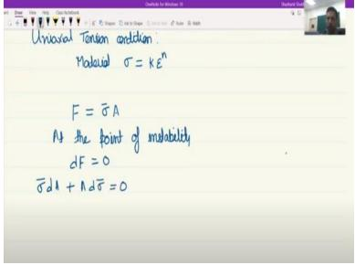
And let us assume that the material has a power law hardening behavior. So  $\sigma = k\varepsilon^n$ . Now we know that let us say we are applying a load F then in the gauge area F is equal to sigma where sigma has to be effective stress times cross sectional area A. Now at the point of instability we know that dF is equal to 0. But we know F is sigma times A. Therefore, we can write it as
