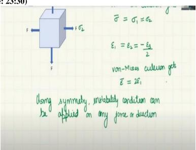
Now using symmetry we can apply the instability condition on any of the forces. Apply it on any force or direction.
