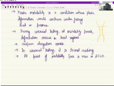
So what is plastic instability? This plastic instability is very obvious particularly when we are doing uniaxial tensile test. So when we see plastic instability and the uniaxial tensile condition, then we see that the load starts to decrease even though the strain is increasing. So we are talking as in terms of the overall component and not as the local stresses.
