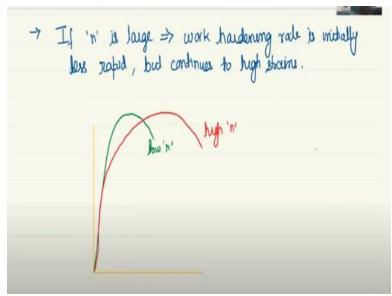
So initially it is less rapid but continues to rise. So if I were to schematically draw this, this is how it would look like. So this is for low n and for high n this is how it would look like assuming that it has almost same elastic constant. So this would be the difference between low n values and high n values. And it is clear why it should be so. Because for high n it means, uniform elongation is high and total elongation is high.
