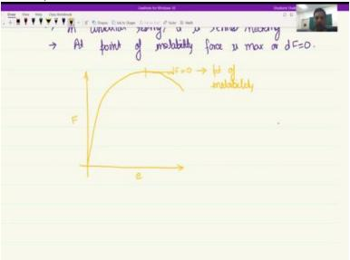
So let us say we are drawing the four, the load versus elongation plot. Then it is at this point where dF is equal to 0 is the point of instability because even though your overall force is decreasing, but elongation keeps on happening. So let us try to understand this with respect to one of the simplest condition which is the uniaxial tension condition.
