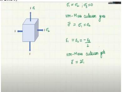
Now let us understand this with the help of one example, which is also similar type. Here it is given to you that the force condition is biaxial in nature and it is balanced, meaning both the forces are same. So if it were  $\sigma_1$ this is  $\sigma_2$ . Then what it is saying is that  $\sigma_1 = \sigma_2$  and  $\sigma_3$  is equal to 0 because it is biaxial, okay.
