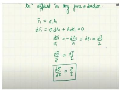
So we have  $F_1 = \sigma_1 A_1$  and again we know that for instability dF<sub>1</sub> it should be equal to which is equal to
