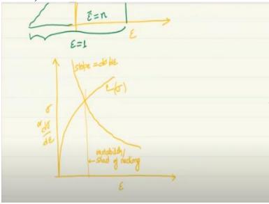
So let us say we are drawing the slope. So the slope is continuously decreasing as you can see, the slope is continuously decreasing, which is represented by this and this is the stress curve. So at one particular point they will intersect. So the slope is equal to d sigma by d epsilon. This is sigma and this is the point where instability or necking starts. So y axis represents stress and also the slope  $\frac{d\sigma}{d\varepsilon}$ .
