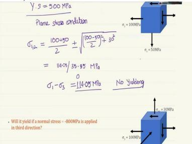
Let us say you are given the stress analysis of a space one of the particular component in a stress graph is given and you are given that the yield stress of the material is 500 Megapascal. So first let us write it yield strength = 500 MPa now you are given the stress state for that component and assume that it is the same everywhere like this. So you have 100 MPa acting here in the x-axis and 50 MPa acting normal stresses along the y axis and there is a shear stress of 30 MPa.
