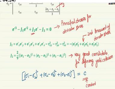
So this would give you the principle stresses for deviator stress where J  $_2$  is the one that. We are interested in so J $_2$  going from this previous equation would look like would have this form and I have already written the equation. So that there is no error in when I am writing it down so J $_2$  would look like this in terms of  $\sigma$  (x, y, z) or in terms of principle stresses. It would look like this where remember
