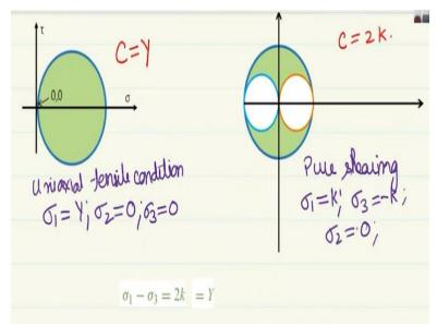
So one of the conditions that we can utilize is again the uniaxial tensile condition and we know that in the uniaxial tensile condition  $\sigma_1 = y$ ,  $\sigma_2 = 0$   $\sigma_3 = 0$ . Therefore when you put it over here we get y - 0 = C and therefore the value of C = y. Now like previous time we will also try to find this constant in terms of the shear strength of the material.
