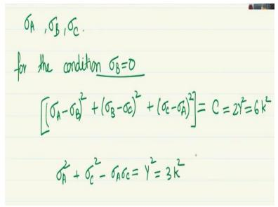
Let us use the term sigma a sigma b and sigma c and here let us say for the condition sigma b=0. How does the plot look like so if you write the so all you have to do is in the sigma equation that we have over here in terms of sigma 1, 2, 3 you can see it is symmetric with respect to  $\sigma$  1, 2, 3 as long as it is in this form of the equation here. It is say that sigma we will now convert it to  $\sigma$  - a, b and c.
