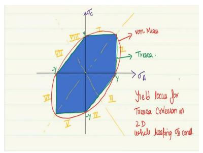
So let us say this becomes your sigma a this becomes your sigma C now we will also draw 45 degree line that is x equal to which will be at equal slope x = y. So it will look like this so anywhere over here sigma C is greater than sigma A and over here sigma A is greater than sigma C. Similarly we will draw a line here because these would define different zones we will get different values or different forms of the same equation.
