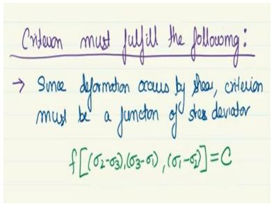
And therefore let us based on our understanding we can say that the Criterions must fulfil the following requirements. What are these requirements let us see, since deformation occurs by shear stress? So, earlier we said that it should be some function of  $\sigma_1$ ,  $\sigma_2$ ,  $\sigma_3$  or  $\sigma_x$ ,  $\sigma_y$ ,  $\sigma_z$  but now we can refine it further. Now we can say since deformation occurs by shear criterion must be a function of stress deviator.
