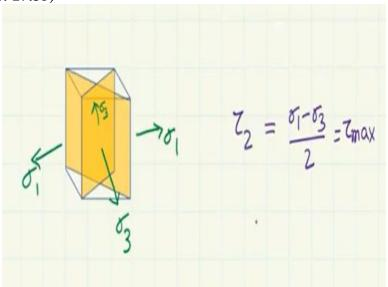
The other condition that we can have where this is sigma 1 and now let us in this particular plane. So, this is so there is a sigma 3 in this direction. So, sigma 1 is in this direction and  $\sigma_3$  is in this direction. So, again for this particular plane the maximum shear stress would be along these orange planes which are at 45 degrees and since  $\sigma_3$  and sigma 1 are the maxima minima and maximum.
