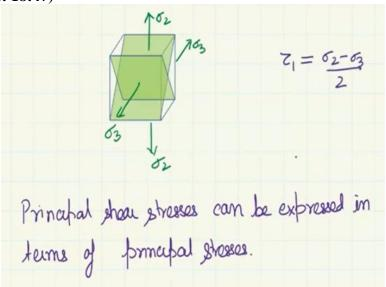
And now over here we have sigma 3 sigma 2. So, here we have  $\tau_1 = (\sigma_2 - \sigma_3)/2$ . And these are the maximum shear stresses in that particular plane so, this is the maximum shear stress in the plane of  $\sigma_{12}$  which is given by  $\tau_3$  is  $\sigma_{12}$ . If you take at any other plane then it would be
