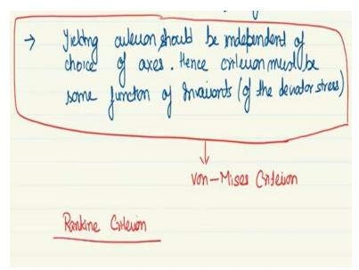
Therefore, the yielding criterion should be independent of choice of axes and hence this something which is independent of the choice of axes is invariant. And therefore, we can also say that this criterion must be some function of invariance and this time not the invariant of the original stress tensor. But now that also, we have described that only the deviator contains the shear stresses so, invariance of the deviator stress component.
