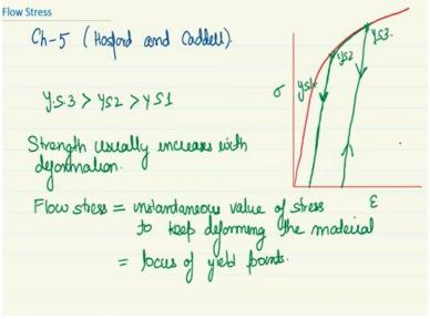
Welcome back students so we will continue our transition to theplasticityofmaterial this part of the content. So far, we have seen the Elastic behaviour we have seen the Tensile properties, Tensile testing, the UTM now we will move on to the plastic behaviour of the material. So, with respect to that first let us get acquainted with the concept of flow stress this content has been covered in chapter 5 by Hosford and Caddell.
