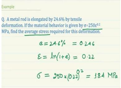
So in this respect let us try to solve one example so the question is a metal rod is elongated by 24.6% by tensile deformation if the material behaviour is given by  $\sigma = 250\varepsilon^{0.2}$ . Megapascal find the average stress required for this deformation. So we what we are given let us take a look at that so you are given engineering string so you are given e which is equal to 24.6% and if you translate it, becomes 0.246.
