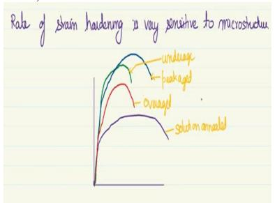
Now this strain hardening rate is very sensitive to the micro structure so even one material under different micro structural condition can give you different strain hardening rates. So, rate of is very sensitive to micro structure again let me and let me draw it here. So, if it were annealed let us say we will take the example of aluminium alloys so if it were aluminium alloy which is age hard enabled but if it were in a annealed condition.
