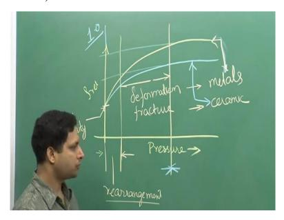
So you need even larger pressure to deform it any further. However one thing you have to keep in mind when we say deformation, this is mostly for metals, what for ceramics? For ceramics actually some amount of fracture will take place even for hard materials some amount of fracture will take place instead of deformation.
