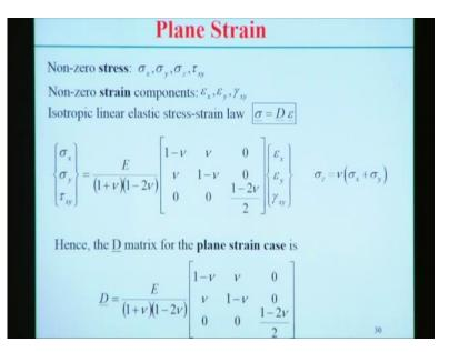
So in general we represents the plane strain condition like this, non-0 stresses are Sigma X, Sigma Y, Sigma Z and Tao XY whereas non-0 strain components are Epsilon X, Epsilon Y and gamma XY. So for isotropic linear (elasto) elastic stress strain law of can be represented, Sigma equal to D into Epsilon; again D actually represents that (po) properties of the materials, but in terms of Young's modulus and the Poisson's ratio.
