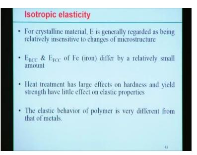
So, there is a few comments on this isotropic elasticity that for crystalline material, E is generally regarded as being relatively insensitive to change of the microstructure, but for BCC and FCC, Young's modulus in case of iron differ by a relatively very small amount. Heat treatment (at) practically having the large effect on the hardness and the yield strength but very little effect on the elastic properties.
