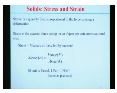
First we define the stress and strain over a solid body. Stress actually quantify, which is the proportional to the force causing deformation to that specific solid. Now stress is actually the external force acting of the object per unit cross-sectional area. So we can measure the stress like that; it is force divided by area that means force per unit area. So unit of stress is in SI it is Pascal or Newton per meter square which is same as the unit of pressure.
