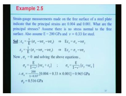
We shift to another problem we can find out that some data which is the measurement from the strain gauge made on the free surface of a steel plate indicate that the principal strain components are point 004 and point 001. What are the principal stresses? Here the assumptions is that no stress normal to the free surface and the values of the Young's modulus and Poisson's ratio for steel are also given.
