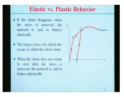
Now, if there is a application of the load in 1 specific direction that is uniaxial direction, then the figure shows the typical stress strain diagram where the initial state from A to B the chord actually follow a linear path but beyond B the diagram becomes non-linear and upto certain point it breaks, that point is called the rupture or the fracture happens at (the) at that point.
