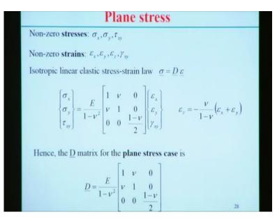
So in plane stress condition, in say we can say that non-0 stresses exist Sigma X Sigma Y and shear stress is only Tao XY and non-0 strains, Epsilon X, Epsilon Y, Epsilon Z and gamma XY. So if we see there are 3 component of the non-0 stresses and there are 4 component of
