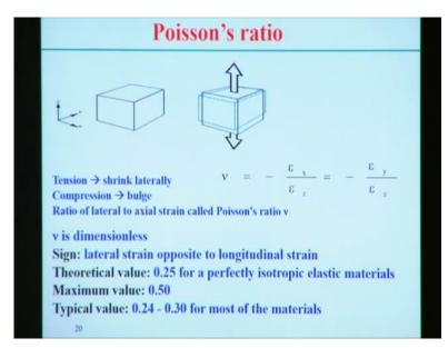
So here, how we can define the Poisson's ratio in this case? The first (())(30:47) indicates the undeformed state but if we apply the load then it will try to deform in 1 direction or maybe extension in 1 direction but other 2 directions probably it can go through the contraction. So, the Poisson's ratio is defined by the lateral strain to the axial strain and that is negative of Epsilon X by Epsilon Z or negative of Epsilon Y and Epsilon Z.
