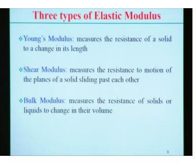
So, 3 different types of elastic modulus is generally we observe in the solid mechanics approach when a material is deformed with the application of some external load. So, 1 is the Young's modulus. Actually it measures resistance of a solid to a change in its length. So, that application of the load here may be either tensile or compressive but in this case the load acts normal to the cross-sectional area.
