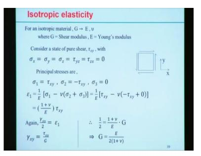
Now let us look into the relation between G, E and Nu, that means between the shear modulus, Young's modulus and Nu; this 3 constant term. First we will try to focus on that, the state of a pure shear condition. So, state of pure shear condition, there exist only one shear stress that is Tao XY, of course with respect to the other components of the other 5, 3 normal stress and 2 shear components as 0.
