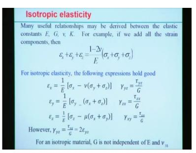
Now, we have discussed there exists 3 different types of (module) modulus as well there are existence of the Poisson's ratio, but using all this elastic modulus or elastic components or we can say elastic constants can find out different correlations among the different parameters. Let us investigate how all these parameters, for example E, Young's modulus, shear modulus, Poisson's ratio, K or D, it is a bulk modulus can also be correlated.
