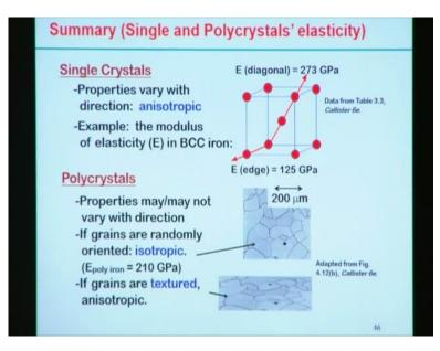
So, in say we can say that for single crystal the properties actually vary with the direction and we know that atomic arrangement of the single crystal is different in different directions, so there is a difference of the Young's modulus at different direction if we look into that picture. So at the diagonal direction, for BCC iron, it is a, the Young's modulus is 273 Giga Pascal, but along the edge the Young's modulus is 125 Giga Pascal.
