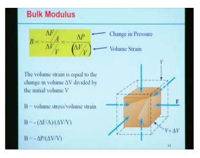
So that delta V with respect to the original V that is called volume strain or volumetric strain and here the bulk modulus is defined by the ratio of change of pressure and the volumetric strain. So the difference from the other 2 modulus with respect to the bulk modulus is that in case of bulk modulus, we representing the stress and strain term acting over the volume.
