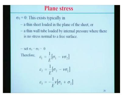
Now if we look into very specific cases; the 3-dimensional state of the stress 1 specific case is the plane stress condition. In this case typically exists when Sigma 3 equal to 0 and practically this happens in case of the things she and when it is loaded in a plane of the sheet or a thin wall tube which is loaded by internal pressure there is no stress on normal to the free surface.
