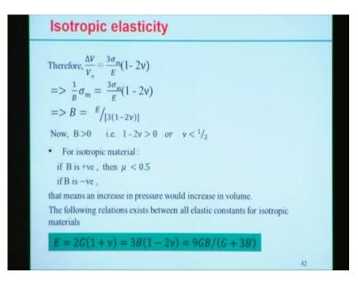
So from this relation we can find out that the definition of the bulk modulus, Delta V by (v) V0 which is equal to 1 by V into Sigma M and right-hand side also there is a Sigma M. So, here we can find out that bulk modulus is a ratio of the E divided by the 3 into 1 minus 2Nu. So these are the expression of the bulk modulus in terms of Young's modulus and Poisson's ratio. Now, if B greater than 0 that means 1 minus 2Nu should be greater than 0 which indicates that Nu should be less than half.
