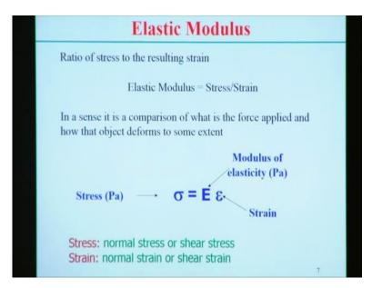
So, within the elastic limit the ratio of the stress and strain is equal to the constant term, that constant term is called as elastic modulus. In the sense that it is a comparison of what force is applied and how the object deforms upto certain extent. So if we look into that expression, the stress is equal to elastic modulus and multiplied by strain. So, since strain is dimensionless, so equation of stress is equal to the here equation of unit of modulus of elasticity.
