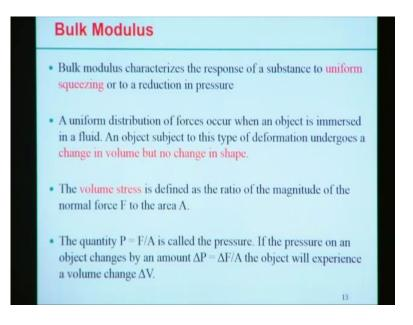
Now, the third modulus that is called bulk modulus which is characterised with the response of a substance when it is subjected to uniform squeezing or is there any reduction in the application of pressure and that actually acts over the volume of an element. So a uniform distribution of forces occurs (c) specifically when the object is immersed in a fluid. And the object is subjected to this type of deformation that is undergoes by the change of volume without any change of shape.
