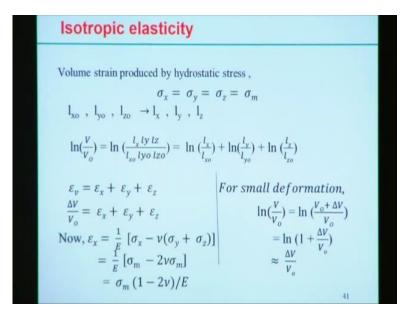
Now suppose volumetric strain actually produced by the hydrostatic stress and in the hydrostatic stress component, the mean stress component is actually called the Sigma X, Sigma Y and Sigma Z. So when there is application of the hydrostatic state of the stress that means (if we) if we consider is as a in terms of pressure, so irrespective of the X, Y and Z, this 3 Cartesian coordinate system all are equal in this case.
