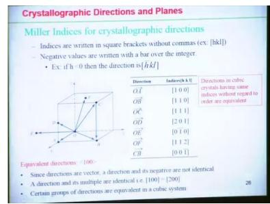
Let us look into the several examples for the Miller Indices of the crystallographic directions. First, first point is that index are written in the square bracket but without commas, that example is given like this, the square bracket and hkl in this form. Next point is that negative values are written within a bar over the integer, but, for example if h less than 0 that means if it is negative then the direction can be represent is like this.
