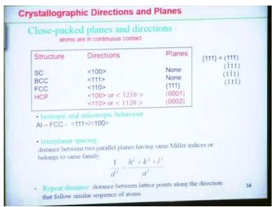
Now, if we look into in the summary that different close packed planes and directions exist in the different type of crystal structure (ob) obviously we have discussed only the simple cubic BCC, FCC and HCP structures. So, among this simple cubic structure, the, we can observe the different close packed planes and different close packed directions. For example; simple cubic structure 1 0 0. So that is the along the edge of a crystal structure that is the close packed direction.
