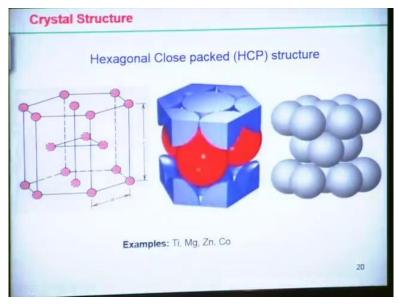
This is one of the most common structure that is called hexagonal close packed structure, (I) HCP structure; here you can see that the that on the face there are 6 atoms exist and the inside the atoms, inside the structure itself there exist the metal layer, 3 atoms again the repetition of the same arrangement on the top surface. So this is the constitution of the hexagonal close packed structure and titanium, cobalt, zinc actually follow this type of structure.
