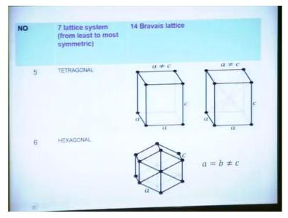
Tetragonal structure is the, where 2 edges are equal but the not the third edges are not equal to others. And it constitute 2 different simple structure as well as body centred structure. Here the hexagonal structure, here (in) in this structure the 2 edges are equal but which is not equal to the height.
