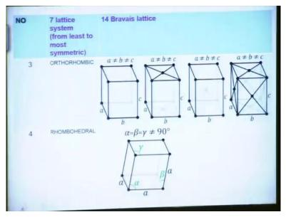
Now orthorhombic structure, in this case which is having 4 different types of structure; simple, base centred, body centred and face centred structure. So here the typical characteristic is that all the edge lengths are not equal but the angles alpha, beta and gamma all are 90 degree. So this constitute 4 different types of orthorhombic crystal structures. Now rhombohedral structure; you are all the angles are not equal but (edge) edges are equal and this constitute only the simple structure.
