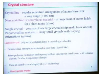
Now we try to shift to the crystal structure of a specific material. So, crystal structure, the next level of the atomic structure where we can find out that the different atoms arranged want a specific sequence. When the regular (re) repetitive arrangement of atoms or ions actually exist over a long range which is typically more than hundred nano meter, then it forms a crystalline structure.
