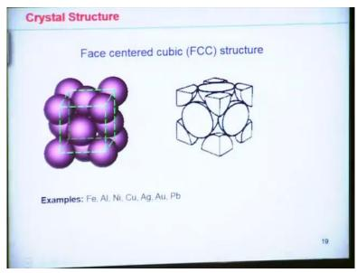
Face centred structure, that is called FCC structure, apart from the 8 cornered atoms there are 6 spaces, on the 6 spaces there exists 6 (diff) atoms also. Iron, aluminium, nickel, copper, silver; these type of materials actually follow the FCC structure. So it is to be noticed that the iron also having BCC structure as well as FCC structure also. So, that we will discuss later on.
