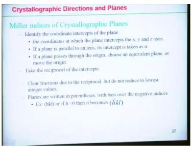
Now we can represents the crystallographic plane in terms of the Miller index form. But in this case we need to first identify the coordinate that intersects on, intercepts on the different axis. The coordinates at which the plain intercepts along the X Y and Z axis need to find out first. If the plane is parallel to an axis then it intercept can be considered as Infinity, if the plane passes through the origin then in this case we can shift the origin or we can consider other equivalent plane.
