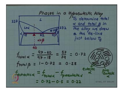
If you wish to do that, then you have to apply, the lever rule just below the eutectic temperature let me draw the diagram. So, this is 18 62 97 alpha liquid plus beta, beta and this is alpha, this is 327 and this is 232. So, we are familiar with this diagram by now, and all I am saying that we are talking of a 40 percent alloy a hypoeutectic alloy and, we want to know what is the total alpha and total beta in this alloy.
