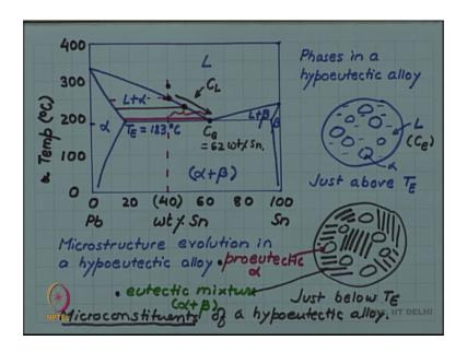
So, we are considering this alloy 40 percent alloy which is our hypoeutectic alloy, the phases in this diagram you are here knowing that is liquid alpha, alpha plus beta liquid plus alpha liquid plus beta and beta.
