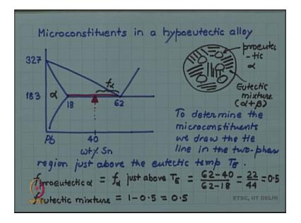
So, let us look at how to determine the micro constituent of the given alloy. So, if you wish to determine the micro constituents. So, remember we had alloy and we had some pro eutectic alpha and, we had eutectic mixture, proeutectic proeutectic alpha, eutectic mixture. So, we can ask for example, that how much proeutectic alpha and eutectic mixture is there in the alloy.
