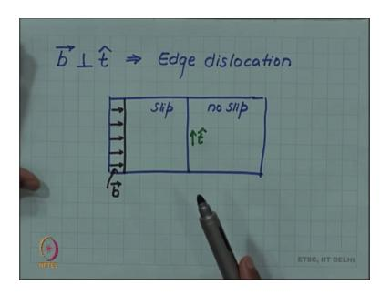
So, in this case we know that for the edge dislocation b and t are perpendicular. So, if b is perpendicular to t, we call the dislocation line and edge dislocation line. So, if we in our slip picture, if we picture it this was the boundary, and when I created a slip from the top view, the first plane went to the position of the second plane, and this was the magnitude and direction of the slip. So, that was b, t of course, is perpendicular so, b and t are perpendicular for an edge dislocation.
