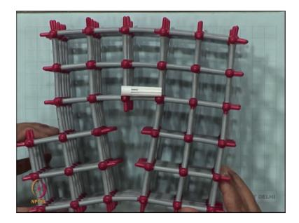
and we said the dislocation line was going in into the page or into your screen. So, it is a horizontal line, which is going into the plane of the drawing, or in this a plane of the model into the model.
