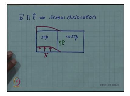
So, if b is parallel to t then the dislocation line is called a screw dislocation, if I again draw that slip plane picture, a slip plane is here, and I want this line to be the dislocation line. So, this side is the slip side and this side is no slip side.
