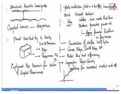
Then the next problem from all infinite domains we went to a structural acoustic waveguide. So, a column of fluid with a rigid plate on the top and a flexible plate at the bottom. We looked at the coupled dispersion curves coupled waves through the coupled dispersion curve. Then we looked at a panel backed by a cavity. So, there is this panel that is vibrating, and it is backed by a cavity this panel vibrates. So, we looked at a paper by Kim and Brennan.
