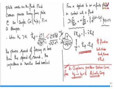
That is the plate works on the fluid and the fluid carries power away on the plate. Now, further at an angle so you get plane waves at an angle  $\cos^{-1}(k_x/k)$  so the fluid is a damper causing radiation damping. Now when  $k_x$  is greater than k then the
