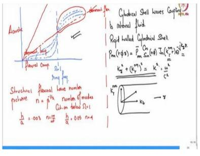
Good morning and welcome to this next lecture on sound and structural vibration. We are looking at this topic of cylindrical shell waves coupling to internal fluid. So, far we have looked at how shell flexural waves behave. So, we have to now bring the fluid aspect in it. So, suppose we have a rigid walled cylindrical shell wall does not move it is a rigid pipe kind of. Then the solution to the cylindrical wave equation has this form let us say
