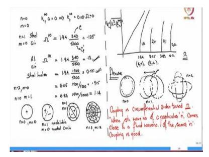
Now based on our table let us look at where the  $k_z$  is cut-on. So, for n = 0 and m = 0 based on the table earlier  $k_r^{00}a$  was 0 which means  $k_r^{00} = 0$  which implies at the same time that the nondimensional frequency  $\Omega$  is 0. Then for n = 1 and m = 0 let us say for steel and air combination my  $\Omega^{10}$  will be 1.84 into c which is 340 divided by 5000. This is speed of sound in the air; this is longitudinal wave speed in the medium; this is about 0.125.
