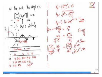
The cut-ons the cylindrical acoustic cut-ons. So, now at the wall the displacement is 0 the normal displacement is 0 which means in the radial direction r = a we will have  $J_n$  the Bessel function first kind n<sup>th</sup> order derivative at r = a shall be 0.
